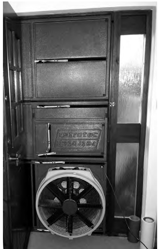
Figure 9.7 Electric blower door for fan pressurization tests
