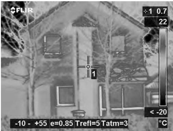
Figure 9.8 IR image of MK1 dwelling; note signs of thermal bridging around the window frames
