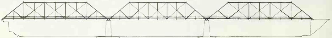
430 Dingmans Ferry Bridge. Dingmans Ferry, Pennsylvania. C.1900. A triple-span Pratt through-truss bridge, built by Phoenix Bridge Co.
