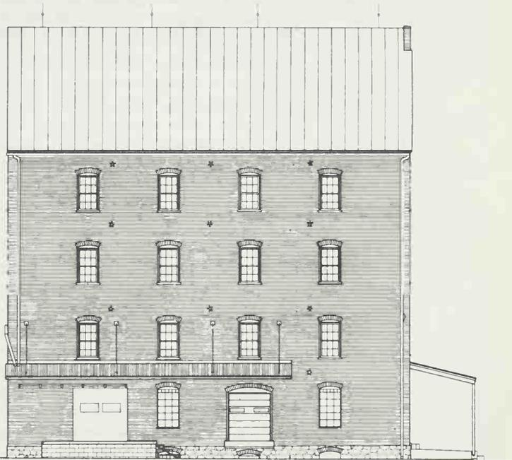
383 Hermann Star Mills. Hermann, Missouri. 1867. A typical steam-powered gristmill. The basement was used for wheat scouring and polishing, the next three stories for milling and flour packing, the attic for dust collection. The concrete loading platform with corrugated metal roof and the garage door are recent additions.
