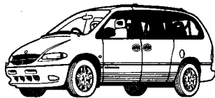
Chrysler Voyager A US people carrier with up to seven seats introduced in the 1990s. Engine options include a 3.3 litre V-6 petrol engine and a 2.5 litre 4-cylinder turbocharged diesel.
