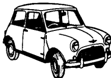
Mini The best selling British car ever made. Designed by Alec Issigonis, the mini was introduced in 1959. Its front-wheel drive, transverse engine, and 10-inch wheels made it an extremely roomy car for its size.
