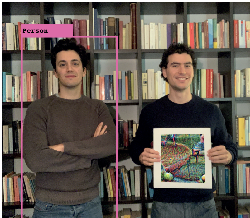
Figure 10.2 Object detection models can correctly identify Gianluca on the left. However, the colorful image held by Nico is specially engineered to confuse the model so it can't detect him.
