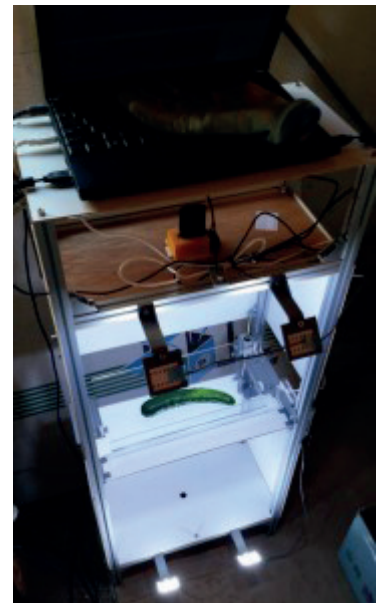
Figure 4.20 Part of the final cucumber-sorting machine, where cameras take pictures of the cucumbers and a computer elaborates the prediction, before moving the cucumber forward, where it's placed in the right bucket.
