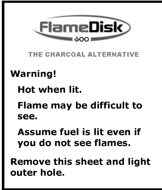
FIGURE 11.2 “Sticky note” warning placed on Smokerplate. This provides an additional layer of safety, conveying essential hazard information and abbreviated instructions even after the film cover has been removed.
