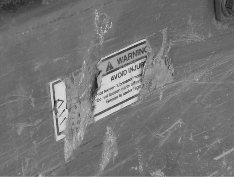
FIGURE 9.9A Warning label rendered useless by abrasion. Labels must be designed, manufactured, and placed to withstand the expected conditions of use for the product.
