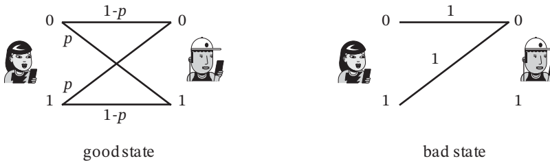
Figure 8.8 Representation of the good and the bad states for a binary channel with binary fading.
