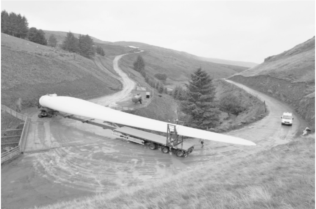
Figure 9.22 One good turn. Delivery of a 52 m blade to an upland UK windfarm using an extended-bed trailer; the access track has been locally widened for clearance. (Reproduced with kind permission of Collett Transport Ltd)
