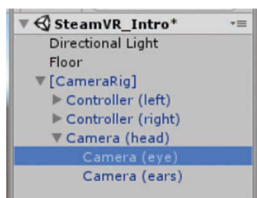
Figure 3.3 Here is the [CameraRig] object with the Camera (head) expanded and the eye selected.
