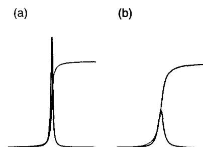
Fig. 2.5 Illustration of how the area or integral of a peak corresponding to a certain number of protons is fixed. The peak shown in (b) is three times broader than that shown in (a); however, they have the same integral (shown by the grey line). As a result, the peak height of the broader line is reduced, also by a factor of three.
