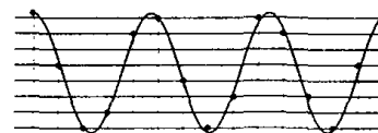
Fig. 12.3 Digitization of a waveform using an ADC with eight levels (three bits). The output of the ADC can only be one of the eight levels, so the smoothly varying waveform has to be represented by data points at one of the eight levels. The data points, indicated by filled circles, are therefore an approximation to the true waveform. Note that the waveform is sampled at regular intervals, as indicated by the grey vertical lines.
