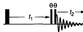
Fig. 10.16 Pulse sequence for the ZCOSY experiment. It is arranged so that only population terms present between the two small flip angle pulses contribute to the spectrum.
