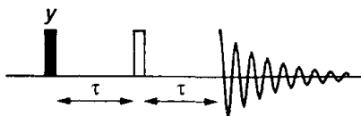
Fig. 7.12 A simple sequence for observing J -modulated spin echoes. The initial 90^\circ pulse about y generates in-phase x -magnetization; a spin echo of total duration 2\tau follows, and then the signal is recorded.
