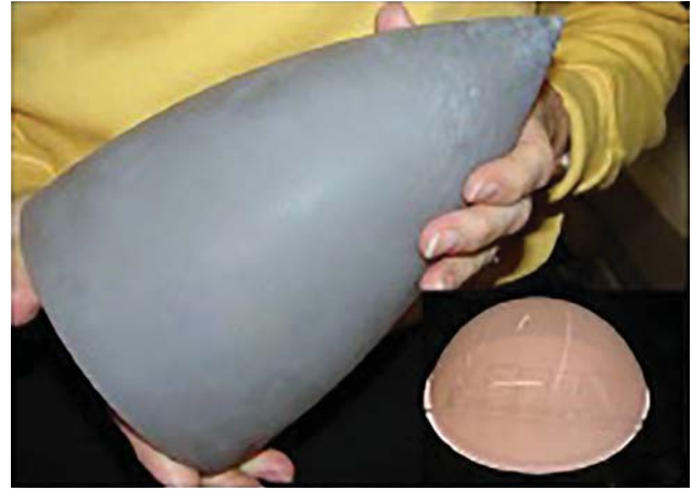
Figure 5.25 IR sensors protective dome made from alumina. Source: Parish and Pascucci 2009 [P9]. Reproduced with permission from SPIE Optical Eng. Press.
