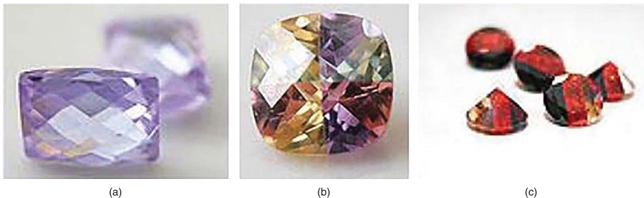
Figure 5.33 (a) Purple, (b) multi-color, and (c) tree-tone cubic zirconia single crystals. Source: Reproduced from https://en.wikipedia.org/wiki/Cubic_zirconia .
