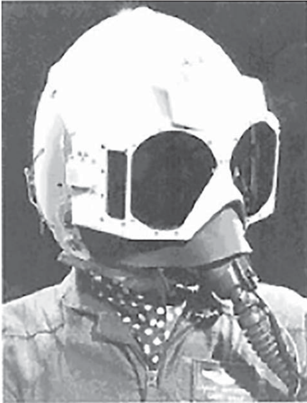
Figure 5.47 Anti-glare goggles based on PLZT plates kept under electric field. Source: Haertling and Land 1971 [H2]. Reproduced with permission from John Wiley & Sons.
