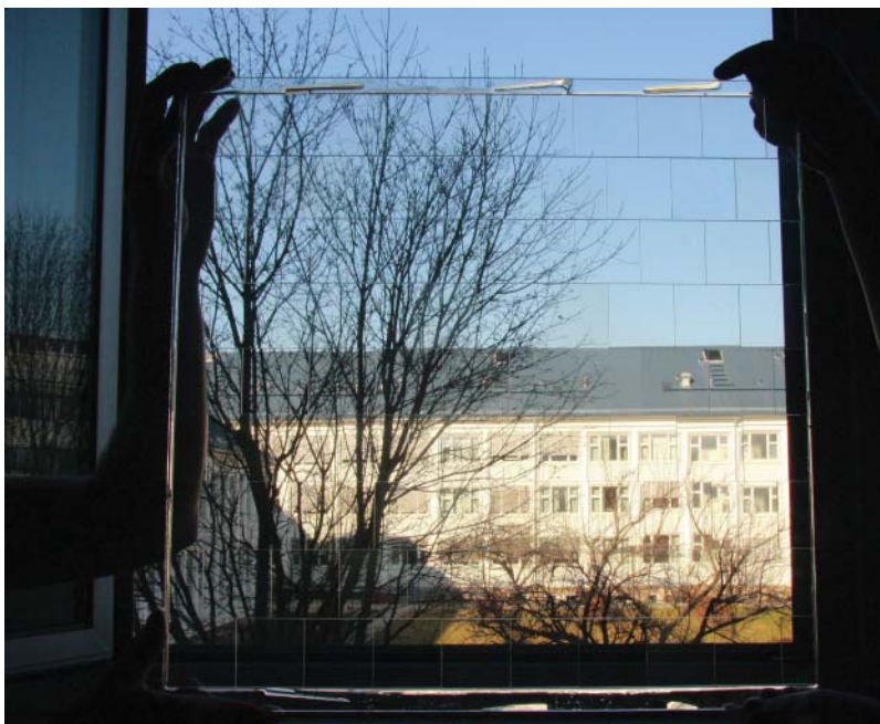
Figure 5.17 Mosaic of transparent Mg-Al spinel tiles with sub-micrometer microstructure on glass backing. Source: Courtesy of T. Hutzler, Fraunhofer Inst.-IKTS Dresden, Germany.
