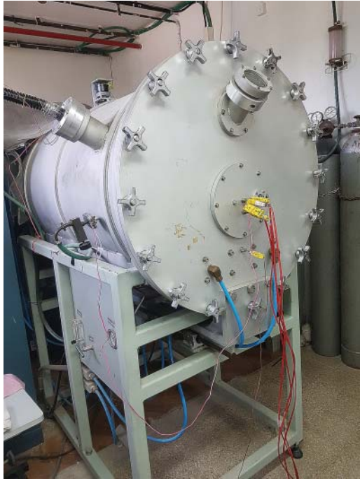
Figure 3.32 Applicator of an MW (2.45 GHz) sintering system (large L/\lambda ratio, multimode operation, mode stirrer Al wall). Source: ICSI, Haifa.
