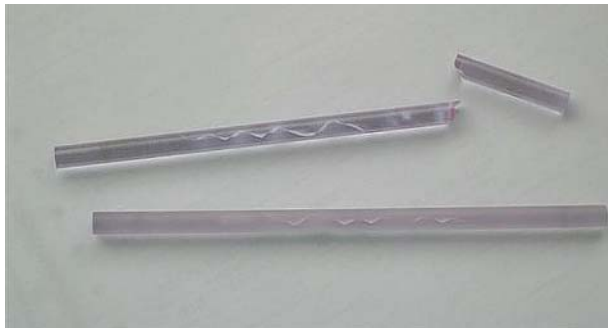
Figure 5.72 Cracking and breaking of Nd:YAG gain media as a result of thermal shock. Source: Courtesy of Feldman [F5].
