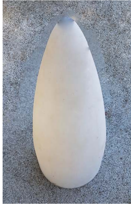
Figure 5.29 Radome (transparent to MW range radiation) made of cordierite crystals based glass-ceramic at ICSI, Haifa.
