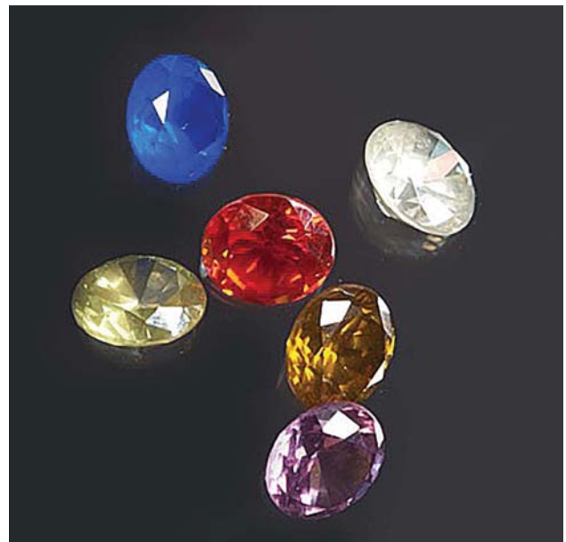
Figure 5.35 Sintered polycrystalline gemstones made of different ceramics. Blue and violet is doped MgAl_2O_4 spinel with a sub-micrometer microstructure, the other four pieces are sintered cubic zirconia ( ZrO_2 ). The hardness HV10 of these sintered polycrystals manufactured by IKTS Dresden is 14–15 GPa for spinel and 12.5–13 GPa for sintered zirconia. Source: Courtesy of J. Klimke, Fraunhofer IKTS Dresden Germany.
