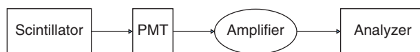
Figure 5.112 Schematic of the setup of a luggage inspection device based on a scintillator type sensor. Source: Adapted from Barta 2012 [B13].
