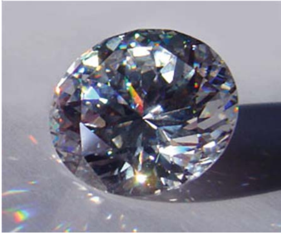
Figure 5.32 Cubic zirconia single crystal, ground and polished as a brilliant (diamond) imitate. Source: https://en.wikipedia.org/wiki/Cubic_zirconia . Licenced under CC BY SA 3.0.
