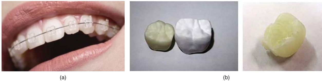
Figure 5.43 Dental products made of translucent ceramics. (a) Translucent alumina based orthodontic bracket. Courtesy of Dr. Ravi Kamiseti, Orthodontic Specialists of Melbourne (OSM), Melbourne, Australia. (b) Presintered stage and finished zirconia made crowns (left panel) and crown made of spinel (right).
