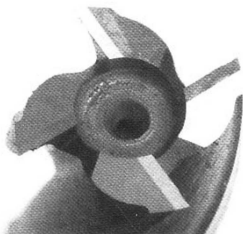
6 View of the end of an end mill showing the end tooth gash.
