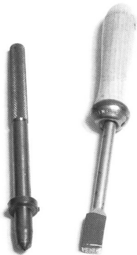
6 Wheel dressers, left single diamond, right multi diamond.
