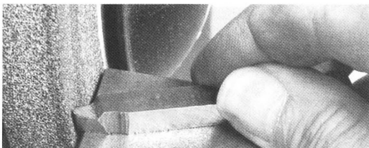
8 Freehand sharpening of the end radius of a round nose tool using a side table extension.
