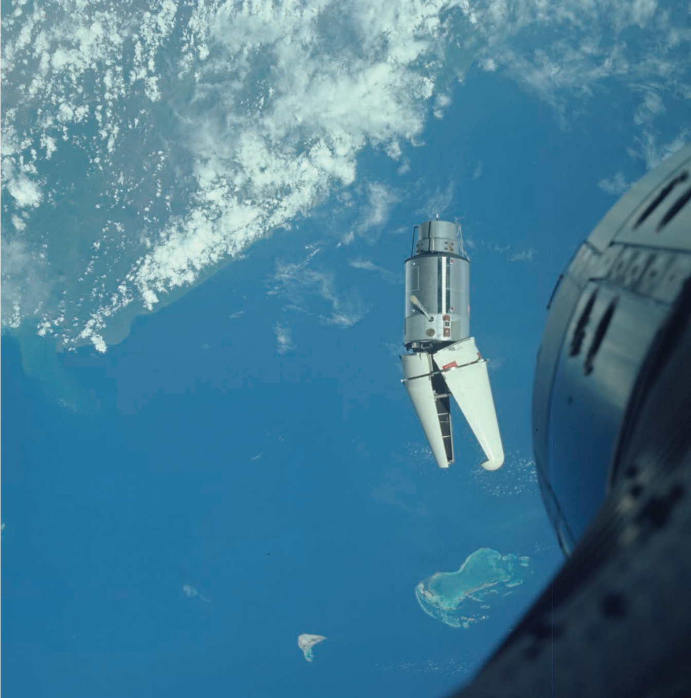
Figure 2.4. The Augmented Target Docking Adapter (ATDA) as seen from the Gemini 9 spacecraft during one of their three rendezvous in space, June 3, 1966, S66-37923 (NASA).
