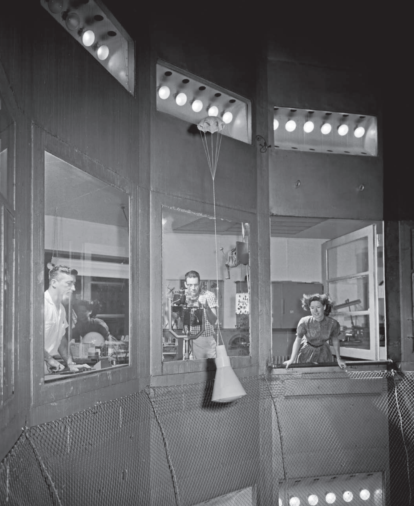
Figure 1.1. Mercury capsule model in spin tunnel at the Langley Research Center, September 11, 1959, LARC Image #L-1959-06212 (NASA).
