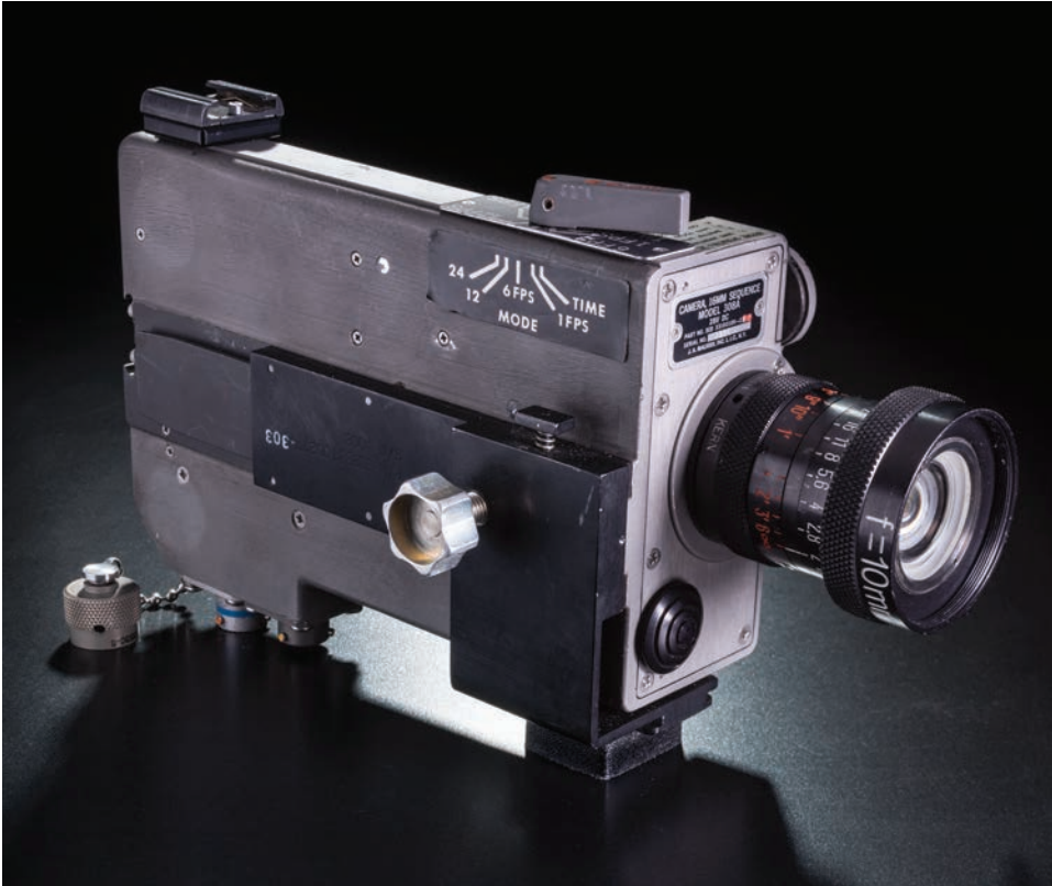
Figure 2.3. Data Acquisition Camera from the Apollo 11 Lunar Module, NASM Cat. #A20190311000 (Smithsonian National Air and Space Museum).
