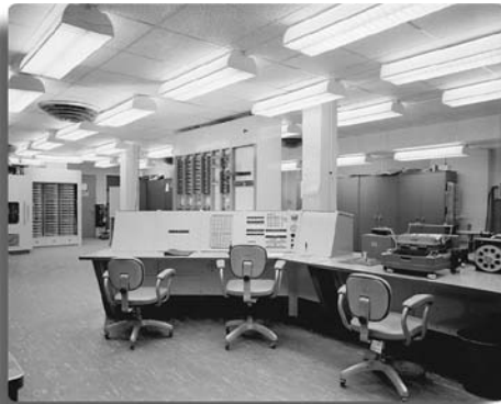
TX-0 transistorized computer at Lincoln Labs, 1956. (Reprinted with permission of MIT Lincoln Laboratory, Lexington, Massachusetts.)
