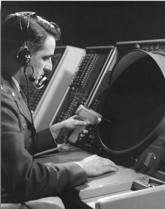
Light gun and SAGE tracking scope. (Courtesy of MITRE Corporation.)
