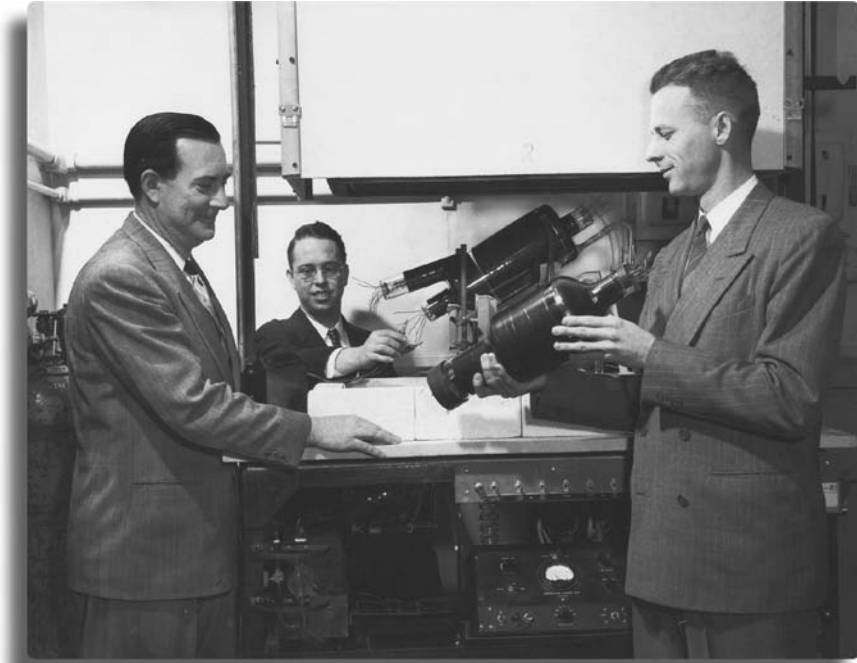
Whirlwind's on-site tube manufacturing department: (left to right)—Pat Youtz, Stephen Dodd, and Jay Forrester examine the finished electrostatic storage tube, 1951. (Courtesy of MITRE Corporation.)
