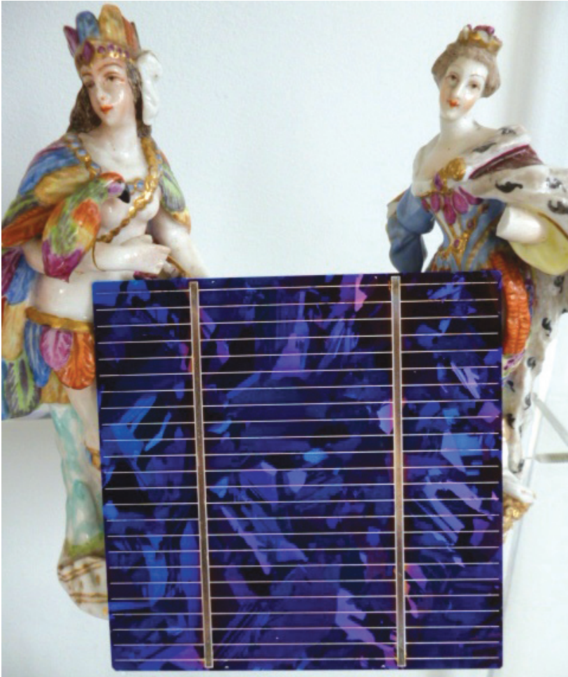
Figure 6.1 A multi-crystalline silicon solar cell (picture by the author).
