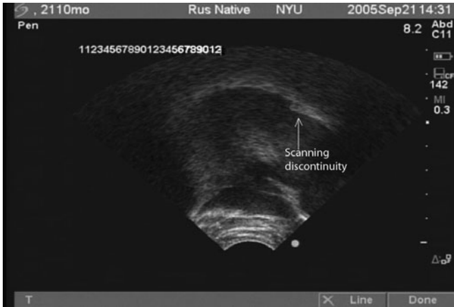
Figure 18.2.2. A scanning artifact in which two different scans of the ultrasound transducer are combined into one image during the production of /n/ by a Russian speaker.
