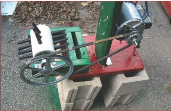
Safety shield installed. Keep hands away from the belt and pulleys!
