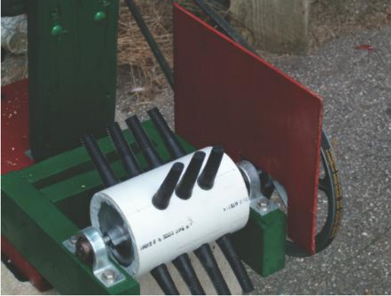
Plucker with belt and tensioner installed.
