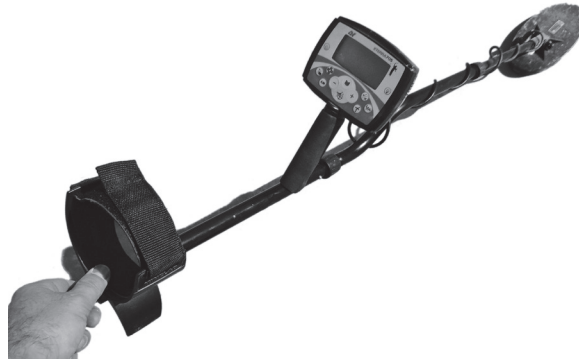
VLF metal detector. Note the cord is securely wound around the shaft to avoid entanglement.
