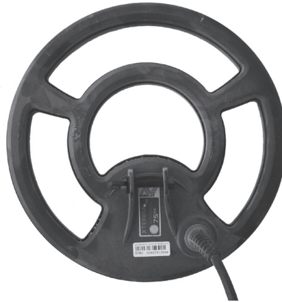
Concentric coil. Note the outer and inner loops for sending and receiving.
