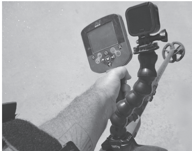
Here is a GoPro Hero4 Session mounted to my detector via a flexible grip mount.
