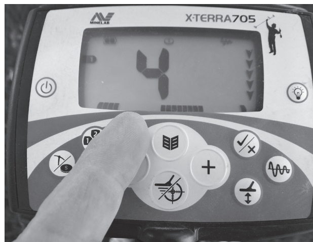
In this example of notch discrimination, the black notches represent targets that have been discriminated, or “notched out,” and the open spaces represent the accepted targets. The author points out the accepted area on this detector.
