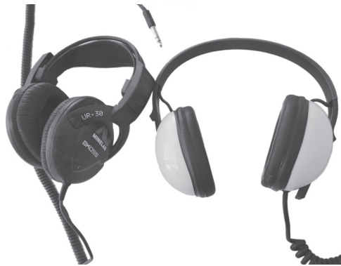
Metal detecting headphones have a wider response, allowing for a broader spectrum of frequencies to be heard.
