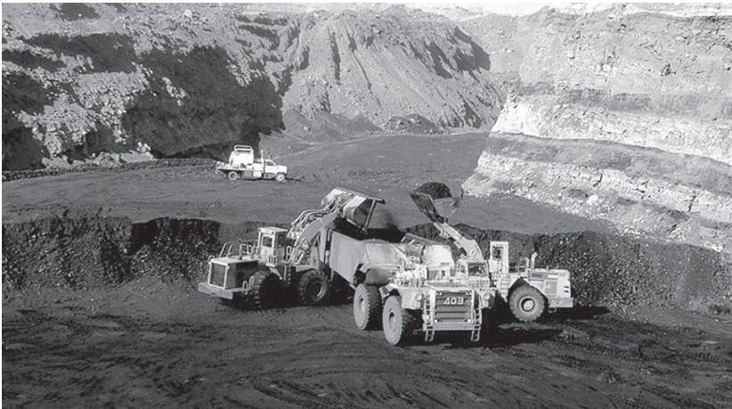
FIGURE 8.7 A photograph of an open cast mine or surface mine. The above picture shows layers of coal being extracted.
