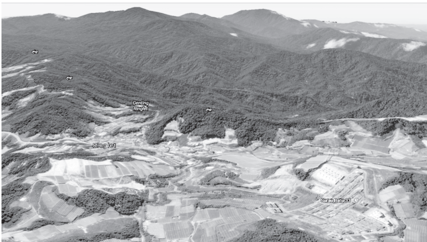
FIGURE 11.4 Google image over Cameron Highlands area in East of Malaysia. This place has experienced many landslides. High spatial resolution and 3D information in the scene allow visual landslide recognition and mapping.
