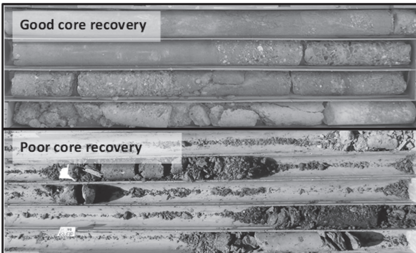
FIGURE 8.10 Core recovery in a diamond drilling campaign for lignite. Good core recovery due to competent rock types (top). The coal and finer and lighter sandy units are missing (bottom).
