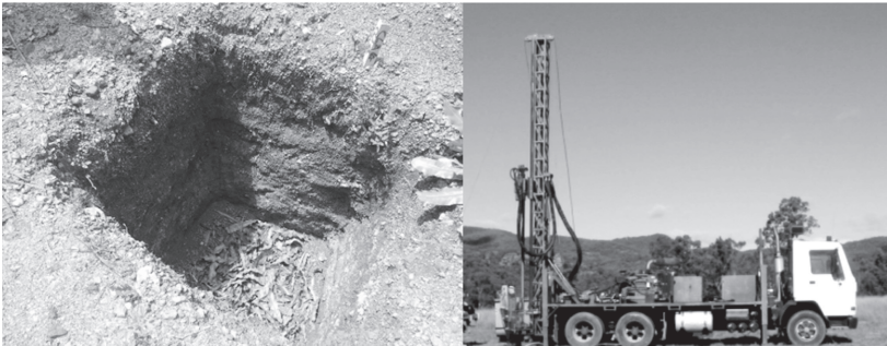
FIGURE 8.4 A trial pit in an exploration project (left). A core-drilling machine at work at a coal deposit (right).
