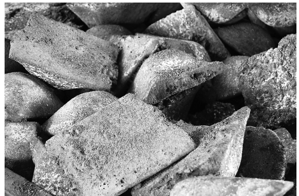
Figure 5.5 Stockpiled Iron Pigs
