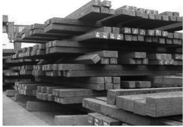
Figure 5.7 Stockpiled Steel Billets
