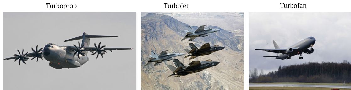
Figure 1.6 Three aircraft engine configurations. There are three main types of engines: the turboprop (propeller), the turbojet (jet), and the turbofan (fan + jet).
