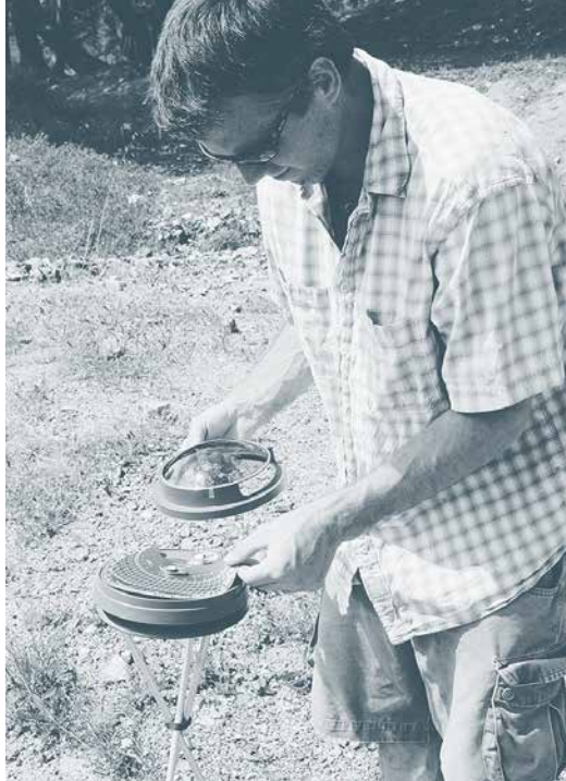
Figure 4.6. Solar Pathfinder. This device allows solar site assessors and installers to assess shading at potential sites for PV systems, helping them select the best possible site to install an array.
