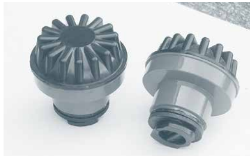
Figure 7.12. Hydrocaps shown here are special battery caps that convert hydrogen and oxygen released by batteries into water, which drips back into the cells of flooded lead-acid batteries, reducing watering. Credit: Joe Schwartz.
