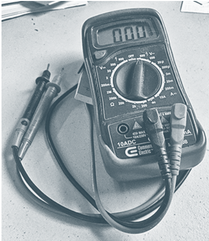
Figure 7.10. Voltmeter for Batteries. Multimeters like these can be used to measure the DC voltage of a battery. You can purchase them at hardware stores and home improvement centers as well as electrical supply houses. Don't waste your money on an analog unit. Go digital! Credit: Dan Chiras.
