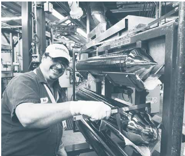
Figure 3.2. Silicon Ingot. This ingot is a huge crystal of silicon that is sliced to make monocrystalline PV cells.
