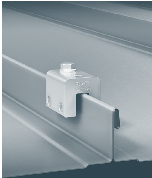
Figure 8.26. Standoff-Mounted PV Array S-5! Clamps. The S-5! clamp shown here allows an installer to attach a PV array to a standing seam metal roof. Rails can be attached to the clamps, then modules can be attached to the rails. Railless mounts are also possible with this mounting hardware. In such cases, the modules are mounted directly to the S-5! clamps, and no rails are used. Credit: S-5!
