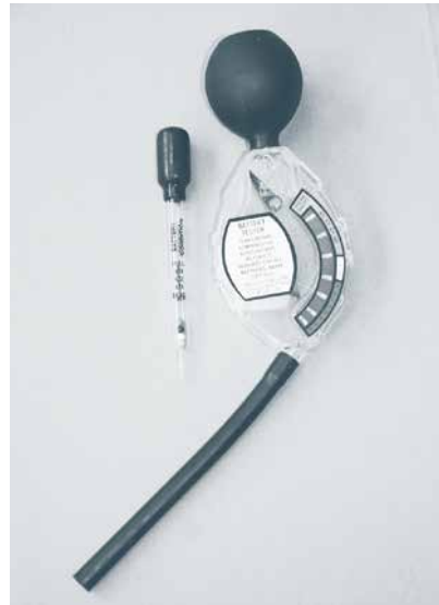
Figure 7.11. Hydrometer. Hydrometers like these can be used to test the condition of battery acid, one cell at a time, a process that is time consuming and boring. They measure the specific gravity, which is determined by the concentration of sulfuric acid, as explained in the text. Be careful when you do this so you don't splash sulfuric acid on yourself. Credit: Dan Chiras.
