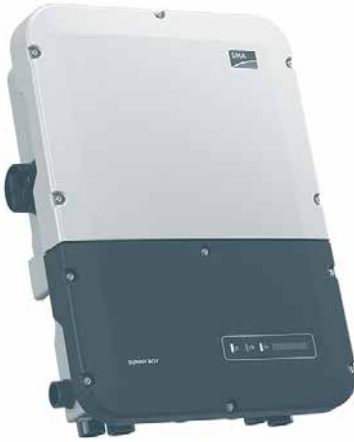
Figure 6.2. This series of inverters ranging from 3 to 7.7 kW comes with an option to add a Secure Power Supply, software and hardware that allows the inverter to continue to produce electricity when the grid goes down. It will send that electricity to an electrical outlet (not shown) attached to the inverter, but not the grid. Total output of the inverter under such conditions is limited to 1,500 watts. Credit: SMA
