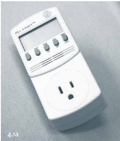
Figure 4.1. (a) The Kill A Watt and (b) Watts Up? meters can be used to measure wattage of household appliances and electronic devices. Of the two, the Watts Up? is the more sensitive and allows for measurement of tiny phantom loads as well. Credit: (a) Dan Chiras, (b) Electronic Educational Devices.
