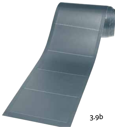
Figure 3.9. (a) PV laminate is applied directly to a standing seam metal roof as shown here. Credit: National Renewable Energy Laboratory. (b) Solar Used for Standing Seam Metal Roof. This photo shows solar laminate, or PVL, from Uni-Solar made from amorphous silicon. This product can be applied on new or existing standing seam metal roofs. Credit: Energy Conversion Devices/Uni-Solar.
