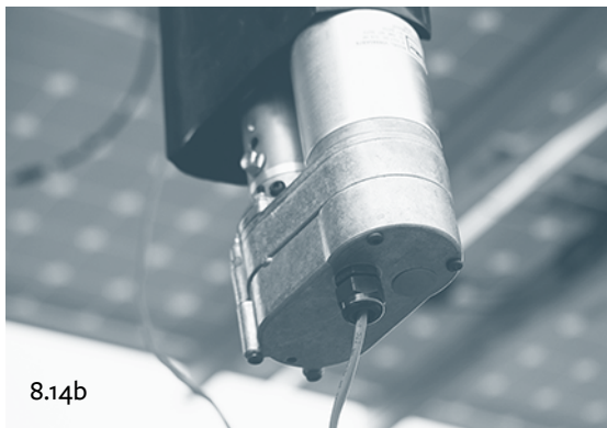
(b) Motor That Adjusts Tilt Angle. A smaller electric motor adjusts the tilt angle of the array to accommodate the ever-changing altitude angle of the Sun. Credit: Dan Chiras.
