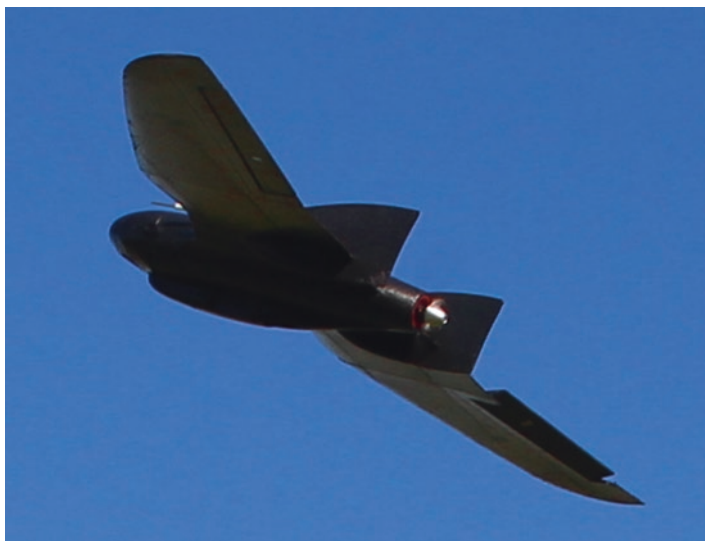
Fig. 2.1 A typical small fixed-wing UAV for scientific and professional applications: the FlyGeo 24 Mpx has a cruise speed of 39 km/h (~24 Mph), an endurance of approximately 30 min, and a total weight of 2.8 kg (6.17 lb). Platforms of this kind can transport a relatively wide range of remote sensors, including visible, near-infrared, thermal, and multispectral devices (Image: FlyTop www.flytop.it )
