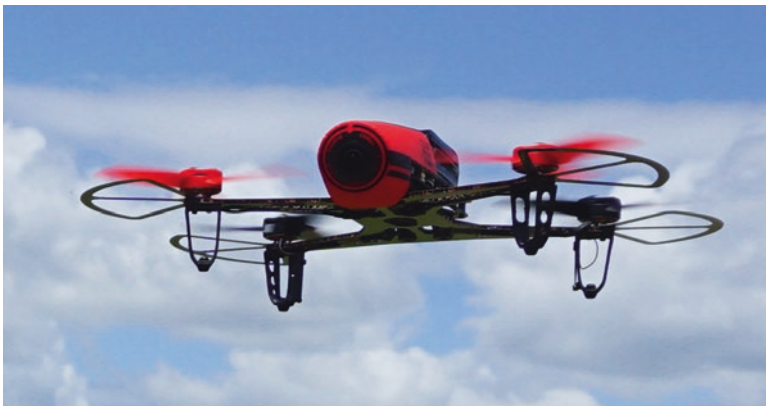
Fig. 2.7 Miniaturization is one of the main development factors for the civilian drone market. While technical performance is increasing, smaller drones are less invasive and easier to deploy. The FTD300X is a custom reengineered variant of the Parrot Bebop drone. Featuring a maximum size of 35 cm and a total weight of 297 g (0.65 lb), it belongs to a category of ultralight commercial micro-drones applicable to observation tasks from video footage to qualitative inspection and aerophotogrammetry (Image: FlyToDiscover)
