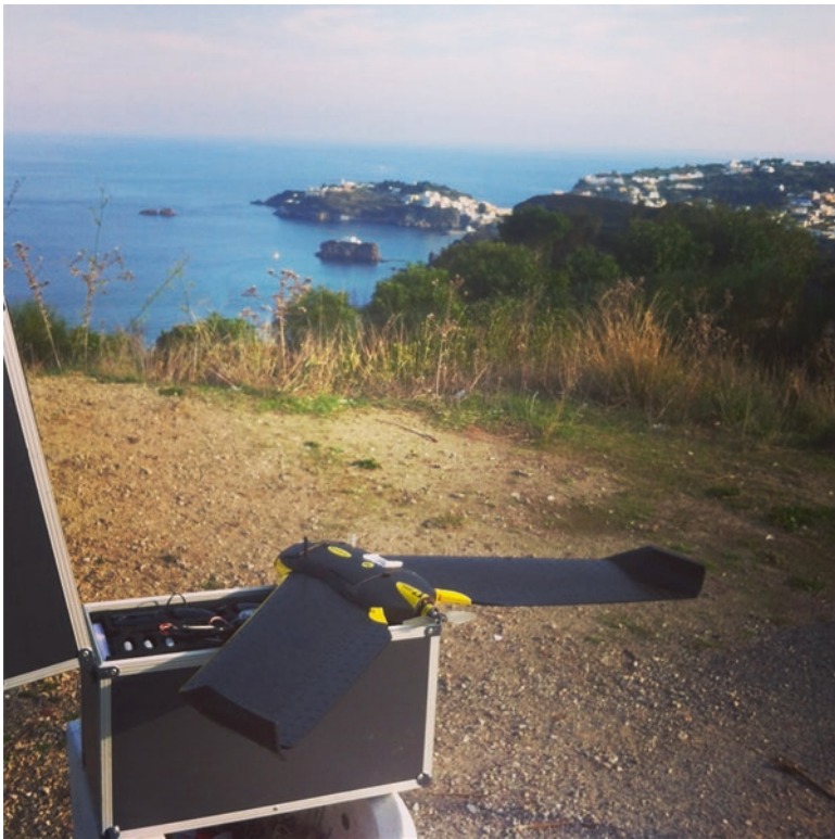
Fig. 2.9 A Sensefly eBee flying wing just deployed on the field, ready for takeoff (Image: Giuseppe Gallo)
