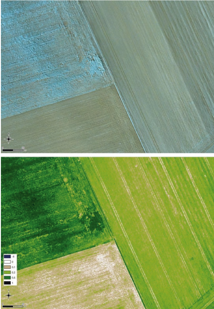
Figs. 3.8 and 3.9 Samples of UAV-based orthomosaics for agricultural research. The image above (Fig. 3.8) is a raw multispectral image taken in the R-G-NIR bands (healthy vegetation in turquoise); the image below (Fig. 3.9) shows calculated NDVI values. The onboard sensor, a Canon A495 camera, was modified to record NIR values by removing the original NIR filter and was replaced by a Kodak Wratten 25 type filter (Image: János Mészáros)
