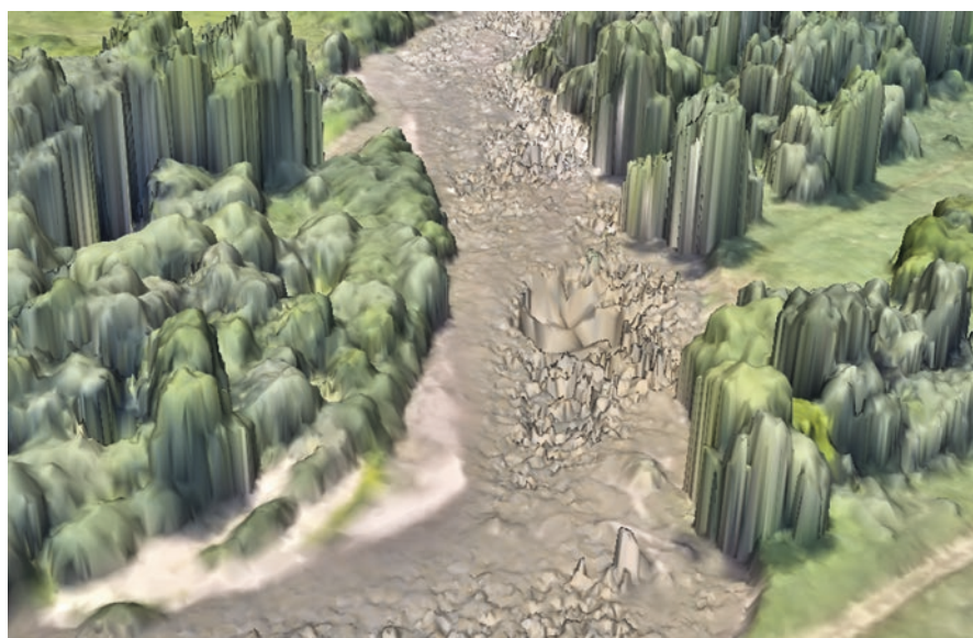
Fig. 4.23 Incorrectly calculated surface in case of stream water
