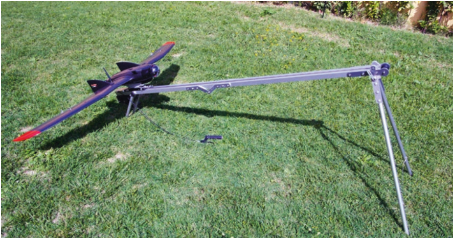
Fig. 2.3 Depending on their size and takeoff speed requirements, fixed-wing UAVs can be launched by hand or by catapults. Drones of this type can land on small spots, either manually or automatically. Below , a FlySecur UAV standing on its field launcher (Image: FlyTop www.flytop.it )
