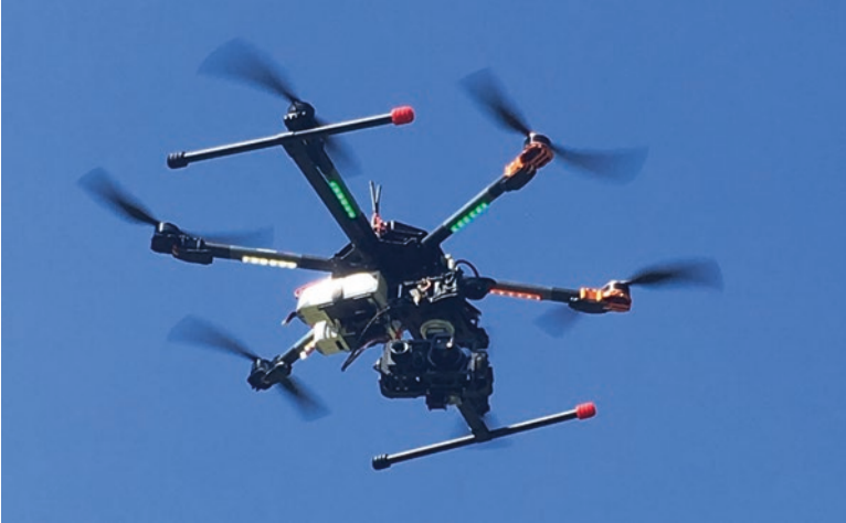
Fig. 2.2 Medium-sized multirotors (above, a 6 kg or 13 lb FlyNovex hexacopter) are suitable for several types of applications spanning from precision farming to detail 3D modeling, to high-profile aerial photo/video documentation. Due to their efficiency and flexibility, they enjoy widespread popularity among professional users, in spite of often severe regulation constraints to their use (Image: FlyTop www.flytop.it )
