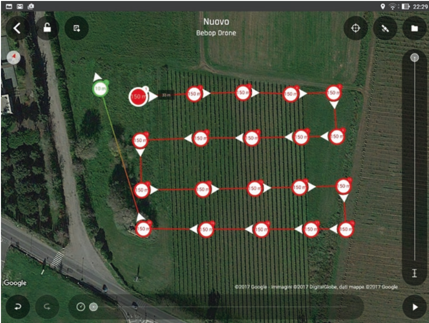
Fig. 4.10 Example of a flight planning interface for UAV mapping (Image: GREAT – European University of Rome)
