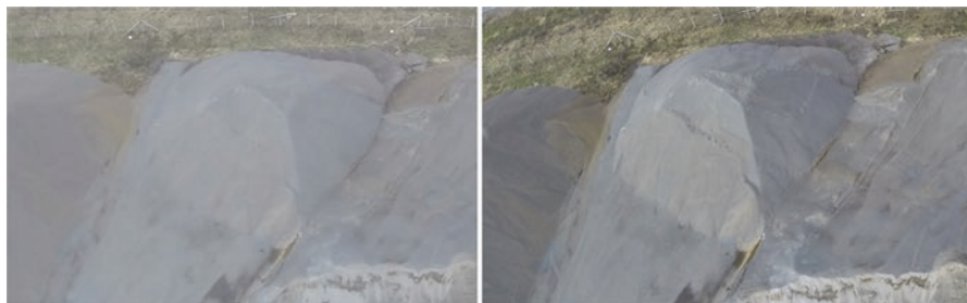
Fig. 4.17 Differences in image contrast in case of cloudy sky ( left ) and clear sky ( right )
