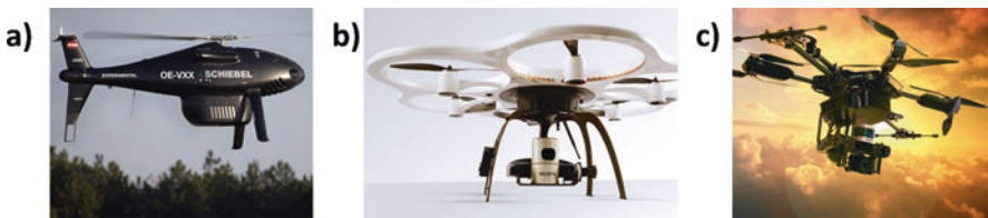
Fig. 4.4 Examples of UAV-borne laser scanners: (a) Riegl VQ-820-GU; (b) Velodyne HDL-32E; (c) Velodyne VLP-16
