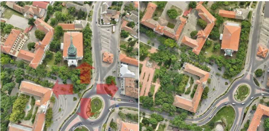
Fig. 4.8 Orthophoto from few largely spaced images with radial distortion ( left ) and true ortho image from a high number of well-overlapping images ( right )
