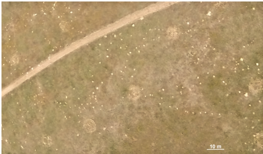
Fig. 4.29 Example of unidentifiable GCP. Among the molehills in the image, it is almost impossible to localize a white, round control point marker
