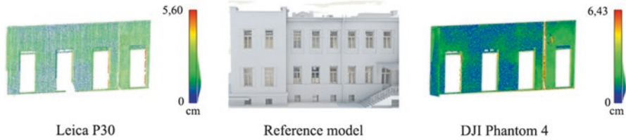
Fig. 5.10 An example of the comparison between the model and the point clouds
