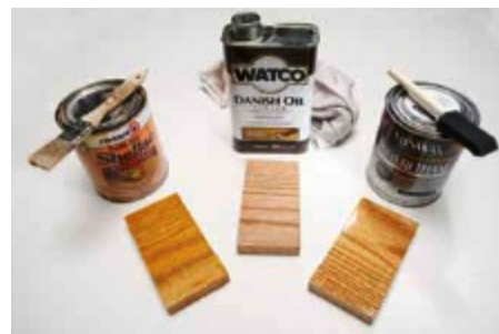
Oak scraps with three kinds of finishes applied. The shellac (left) imparts a mellow orangish tint; the natural Danish oil (center) enriches the grain and offers moderate protection; high-gloss polyurethane creates a shiny, protective coat.
