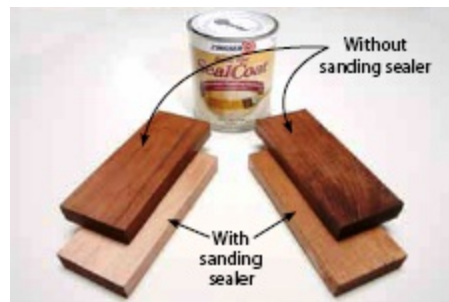
Maple boards (left) and pine boards (right) that have been stained without sanding sealer (top boards) and with sealer (bottom). Sanding sealer evens out the absorption rate to provide a more uniform look.
