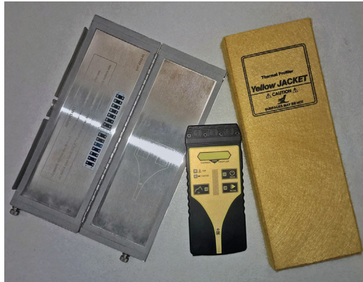
FIGURE 2.14 Traveling solder profile logger with double insulation.
