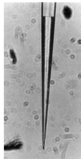
FIGURE 23-10 Photograph of a potassium liquid-ion exchanger (valinomycin) microelectrode with 125 \mu\text{m} of ion exchanger inside the tip. The magnification of the original photo was 400\times . (From J. L. Walker, Anal. Chem. , 1971 , 43 , 89A, DOI: 10.1021/ac60298a780. Reproduced by permission of the American Chemical Society.)
