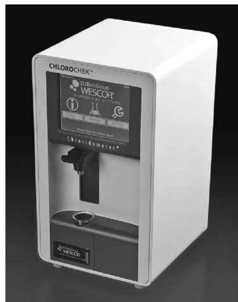
FIGURE 24-11 A commercial digital chloridometer. This coulometric titrator is designed to determine chloride ion in such clinical samples as serum, urine, and sweat. It is used in the diagnosis of cystic fibrosis. The chloridometer is also used in food and environmental laboratories.
