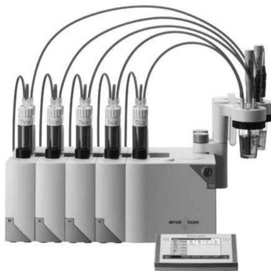
FIGURE 23-19 High-performance automated titrator. Accommodates up to six buret drives, has user-programmable software, permits high sample throughput with an automatic sample turntable (not shown). The unit can be adapted for several different types of titrations. (Copyright 2006 Mettler-Toledo, Inc.)
