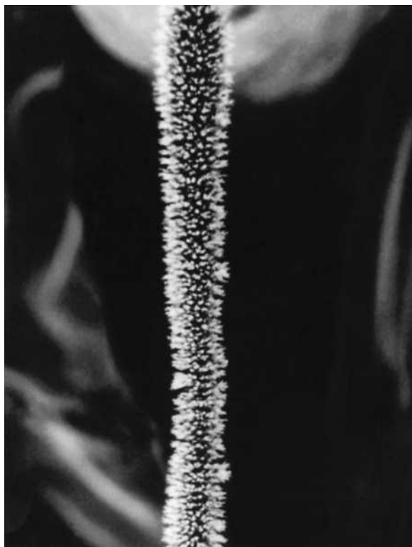
FIGURE 20-5 Photomicrograph of a carbon microneedle emitter. (Courtesy of R. P. Lattimer, BF Goodrich Research and Development Center.)
