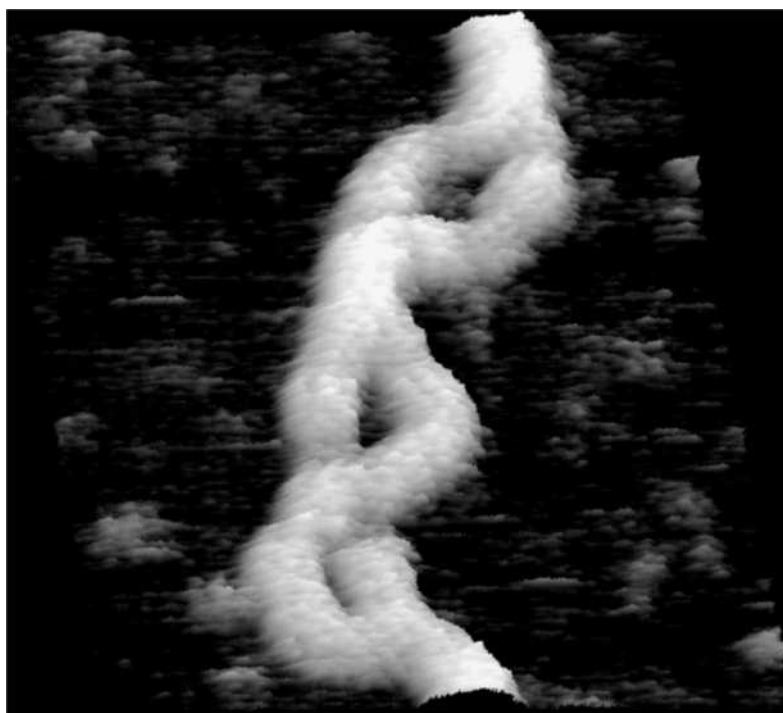
FIGURE 21-30 Two double-stranded DNA molecules imaged on mica, showing the ability of an AFM to resolve overlapping molecules. (Courtesy of W. B. Stine, University of California, San Diego. With permission.)
