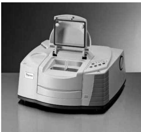
FIGURE 16-6 Photo of a basic, benchtop FTIR spectrometer suitable for student use. Spectra are recorded in a few seconds and displayed on a laptop computer. Software is available for controlling the instrument, collecting and processing data, and analyzing the results. An IR database is included for analysis and spectral interpretation. (Courtesy of Thermo Electron Corp., Madison, WI.)
