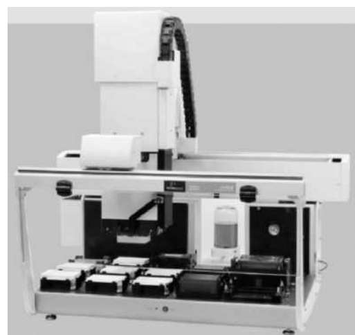
FIGURE 33-16 Automated workstation for dispensing liquids into microtiter plates and deep-well plates. The unit can accommodate 96- and 384-well plates. (Courtesy of PerkinElmer, Inc., Waltham, MA)
