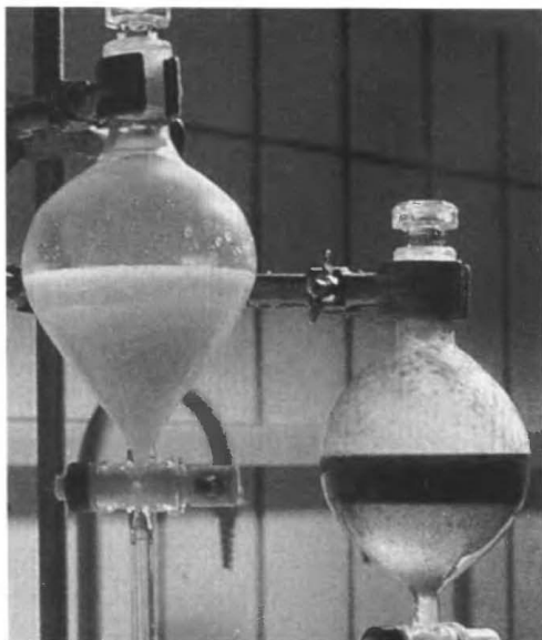
FIGURE 4.3 Emulsion in a separatory funnel compared to a normal two-phase system.
