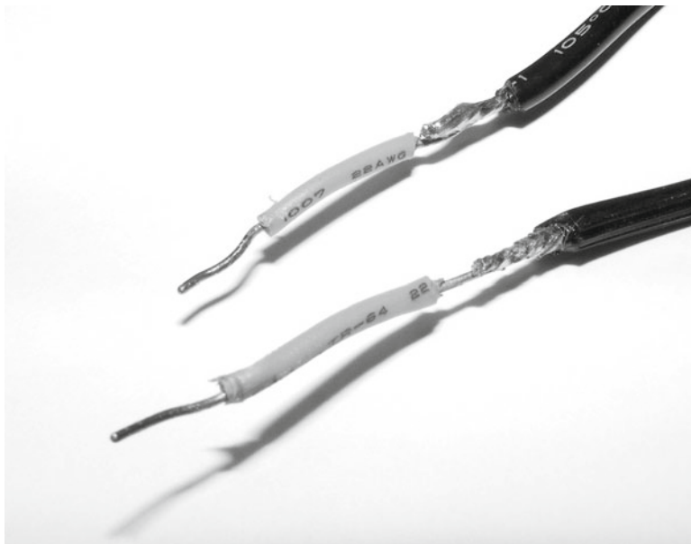
Figure 2-6. Power supply leads with breadboard-friendly tails added
