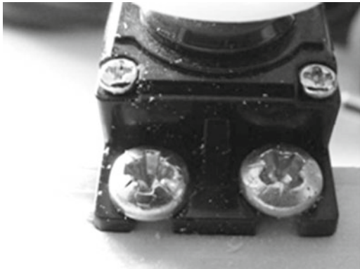
Figure 4-6. Using self-tapping cheesehead screws
