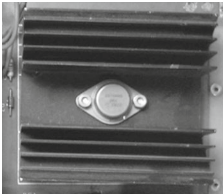
Figure 4-23. 2N3055 transistor on a heatsink
