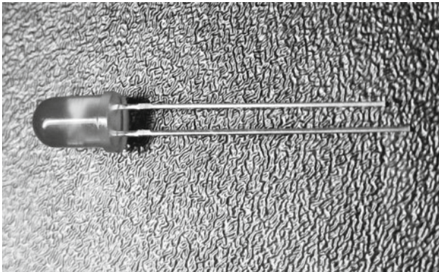
Figure B-9. A single LED - the longer of the two wires is the positive lead
