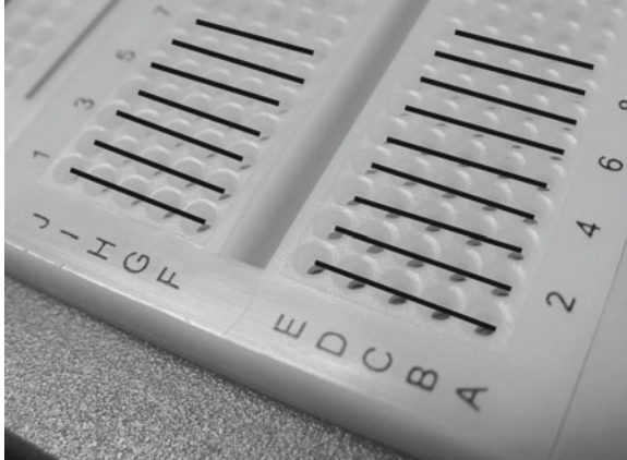
Figure C-2. Interconnected column holes
