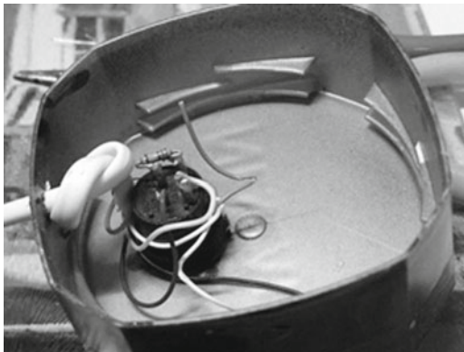
Figure 10-7. The coffee jar lid button mount
