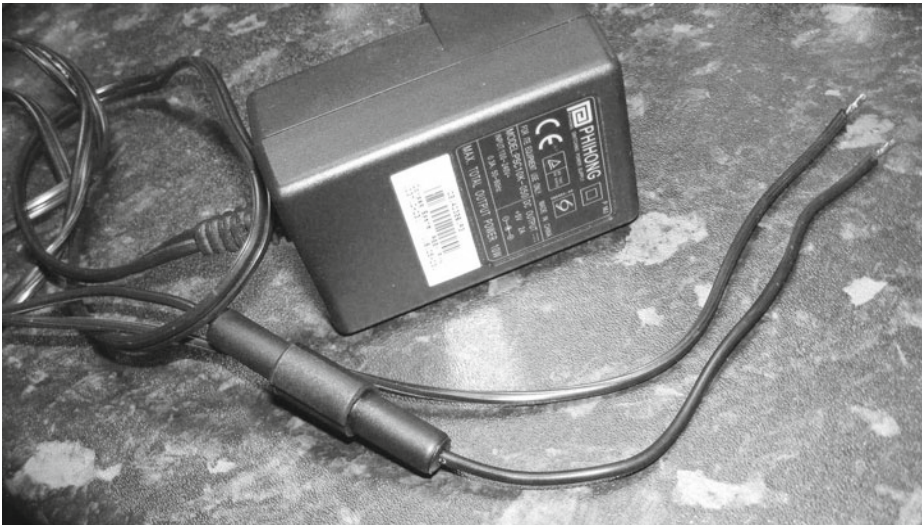
Figure 2-5. A repurposed 5 volt supply
