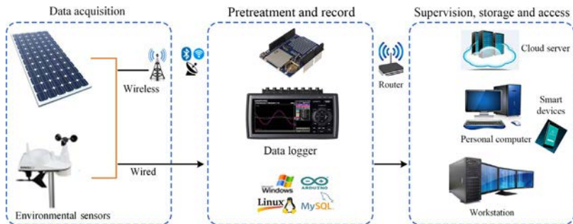
FIG. 5.6 General scheme of a PV monitoring system [28].
