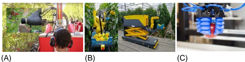
FIG. 7.6 (A) Apple vacuum-harvesting robot, developed by Abundant Robotics [31], (B) Sweet pepper harvesting robot, developed by Sweeper [32], and (C) Robotic grippers and the control unit, developed by Soft Robotics [33].
