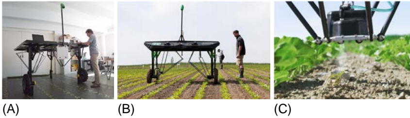
FIG. 7.9 (A) Lab testing of the robot's vision and weed control system [46], (B) the robot working in a sugar beet field in Switzerland [47], and (C) The robot arm placing a microdose at the right spot [45].
