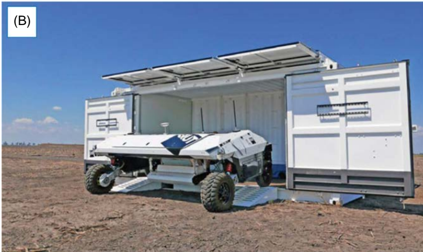
FIG. 7.12 Solar-powered AgBotII weeding robot [50]: (A) Robot's major assemblies, and (B) The robot docking with the solar charge station.
