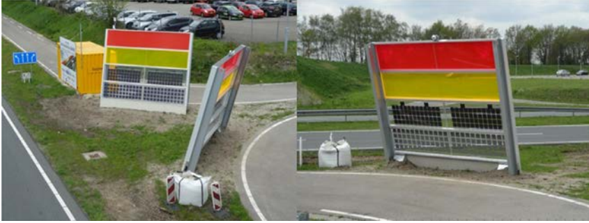
FIG. 11.9 Photographs of the noise barrier prototypes [61].
