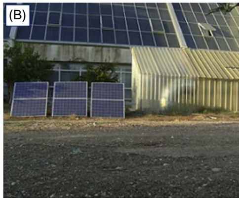
FIG. 6.23 A grid-connected PV-powered cooling system integrated with a greenhouse [110]; (A) Schematic view of the system, and (B) Photo of the experimental setup.
