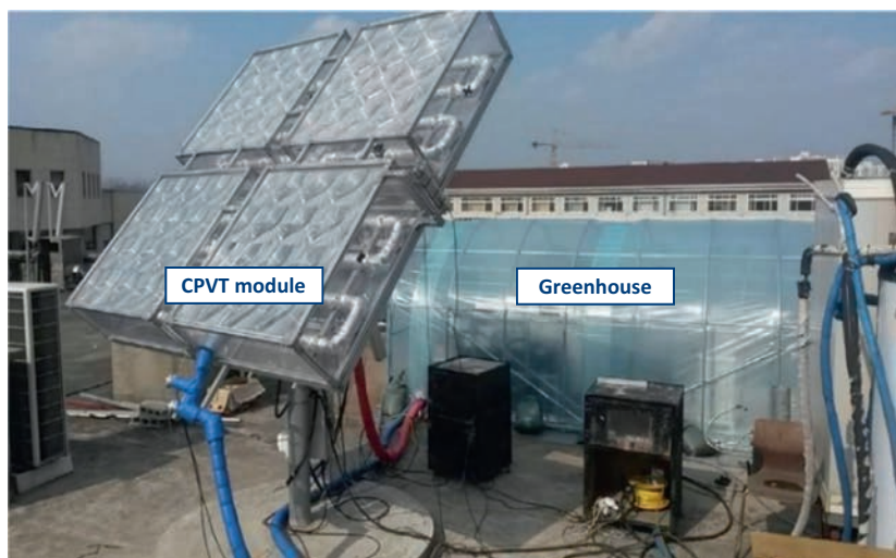
FIG. 6.27 The experimental setup of the greenhouse integrated with a CPVT module [126].
