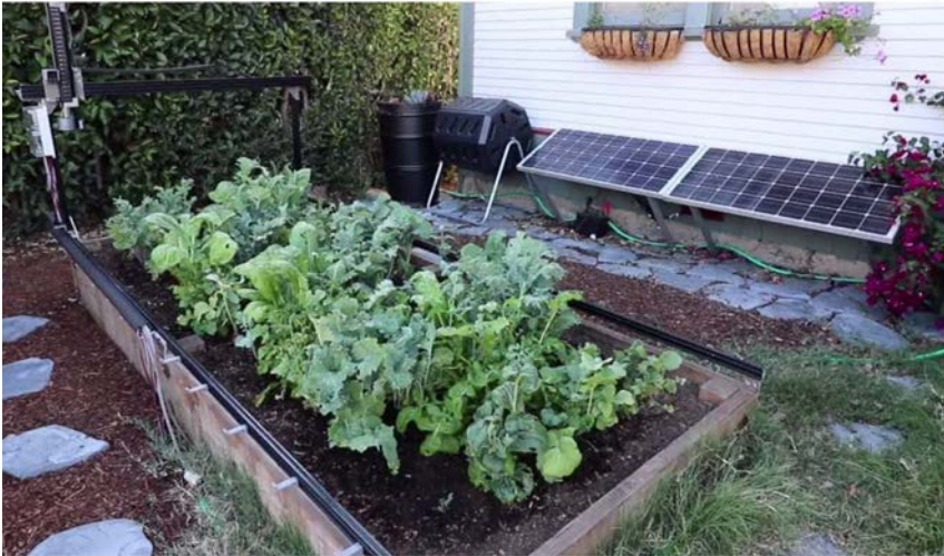
FIG. 7.16 FarmBot precision farming tool [62]: (A) the physical structure, and (B) FarmBot powering with PV modules.
