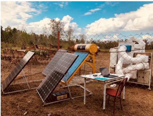
FIG. 6.19 The experimental installation of the solar-assisted drying system developed in ref. [89].
