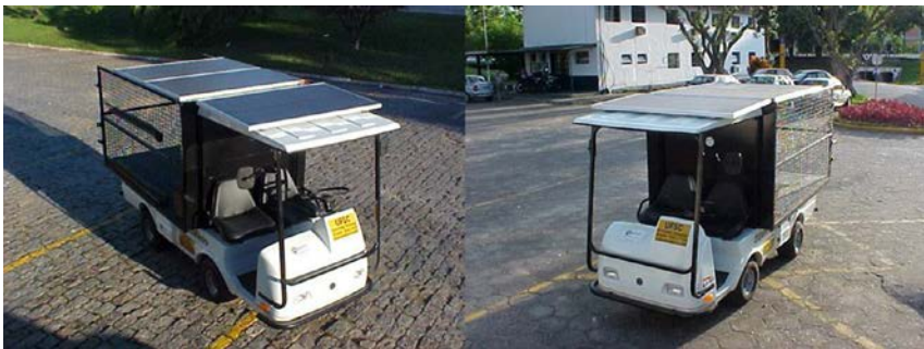
FIG. 11.10 Electric solar quadricycle developed by the Universidade Federal de Santa Catarina in 2003 [66].
