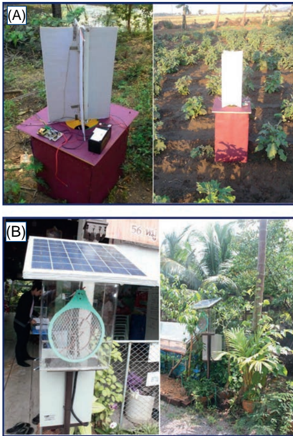
FIG. 6.30 Solar-powered light traps: (A) The model (with funnel) used in the Brinjal field [137], and (B) the model (with electric wire mesh) implemented in a coconut farm [138].
