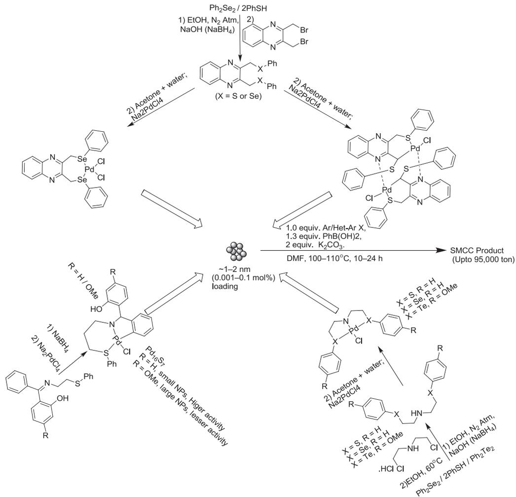
Fig. 8.5 Synthesis of various palladacycles and pincer complexes and subsequent degradation to PdNPs.
