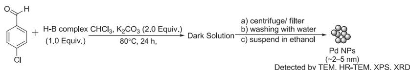
Fig. 8.14 Complete protocol to synthesize HB complex derived PdNPs.
