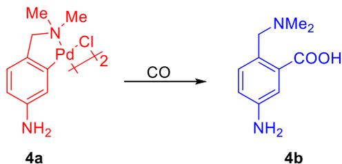
**Scheme 10.4** Carbonylation reaction of palladacycle **4a** on the surface of AuNP.
