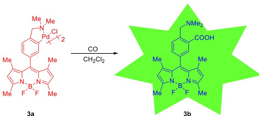
**Scheme 10.3** Fluorogenic carbonylation reaction of palladacycle **3a**.
