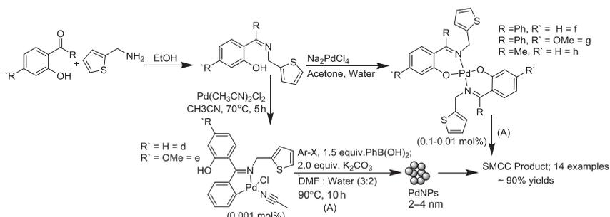
**Fig. 8.8** Synthesis of imine-based ligand and its corresponding palladacycles utilizing different Pd salts thereby giving rise to two different pathways to catalyze subsequent SMCC.
