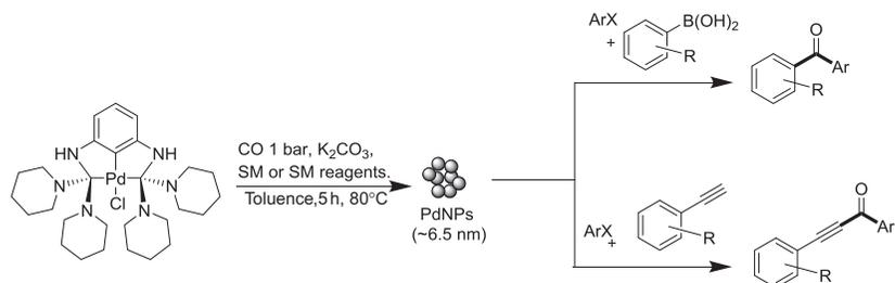
**Fig. 8.17** Degradation of pincer complex based Palladacycle in CO atmosphere to give PdNPs and its first ever subsequent use in carbonylative SMCC and SHCC.
