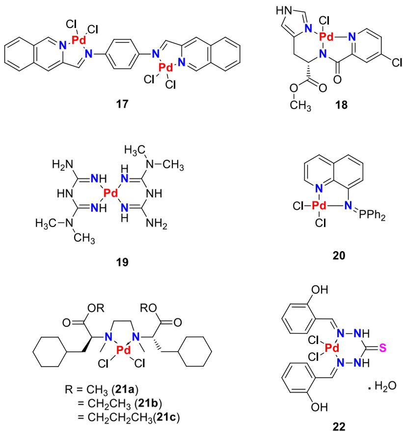
**Fig. 9.6** Palladacycles (**17–22**) bridged by a phenylene ring complex **17**, Pincer type palladium complex **18**, palladium complex benzylamine ligands **19**, iminophosphorane ligand based **20**, R2edda-type ligands **21**, thiocarbonyl ligand with salicylaldehyde **22**.
