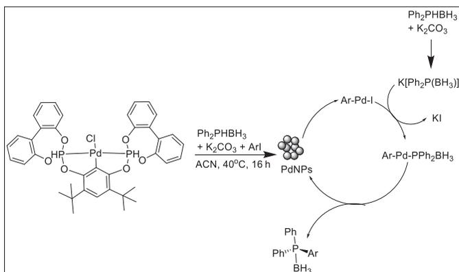
Fig. 8.3 Proposed mechanism for the aforementioned carbon-phosphorous coupling.
