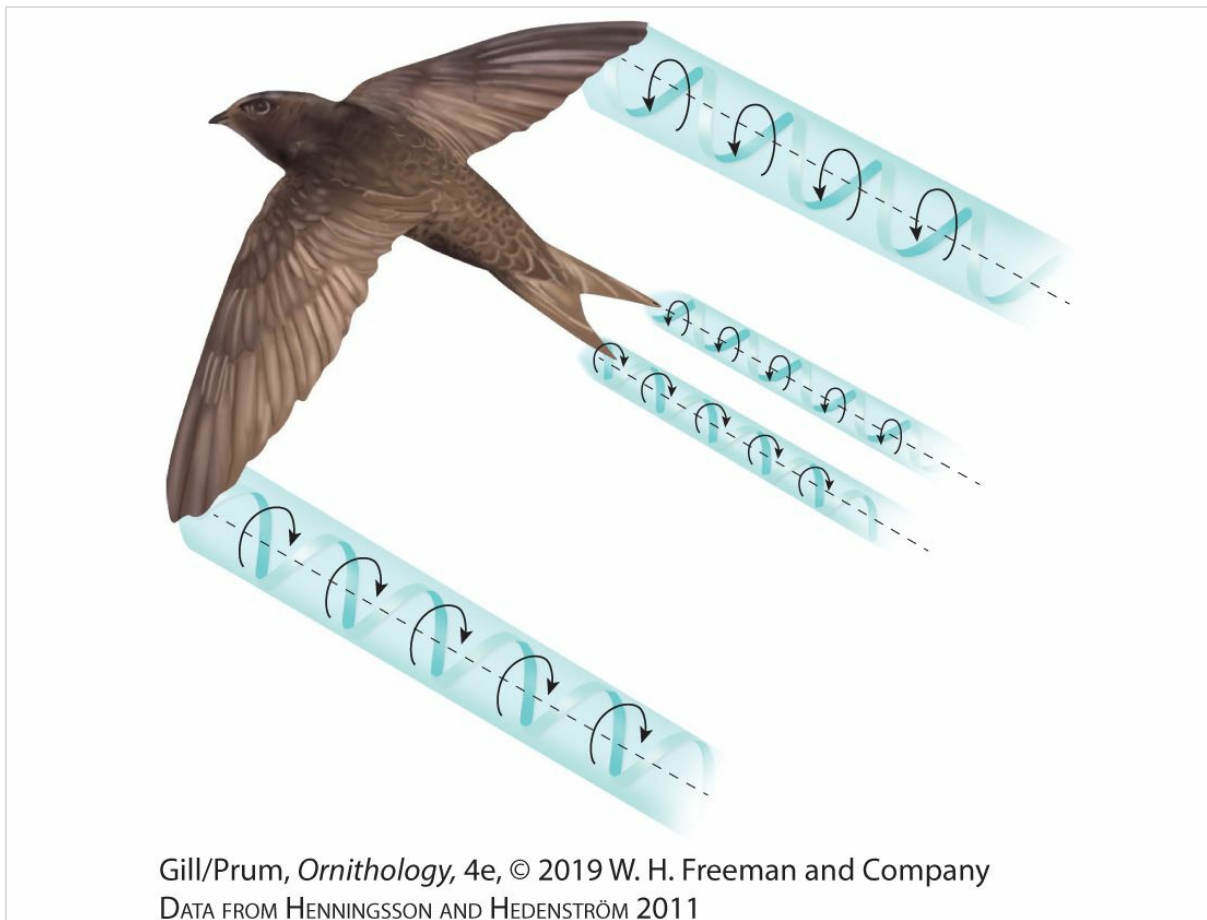
Figure 5–2 As the bird flies, it leaves trailing vortices of circulating air in its wake. The direction of the vortices creates a downwash of air immediately behind the bird. Trailing vortices contribute to induced drag.
