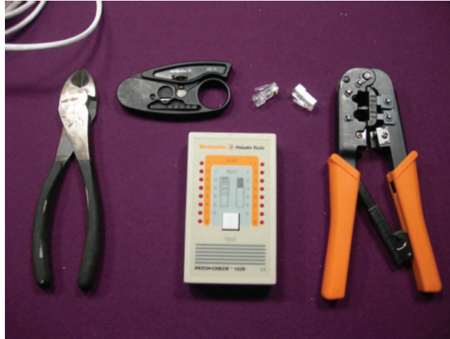
FIGURE 3.4 Patch cable tools
