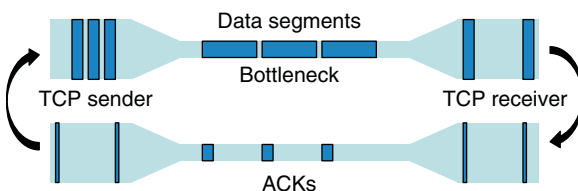
Figure 10.2 Self-clocking mechanism of the TCP connection.
