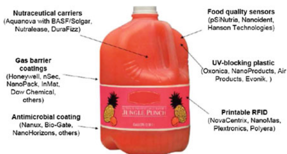
Fig. 17.14 Nanovisions for bottled products. Image courtesy of IoN, UK. Source Lux Research reference study. The Nanotech Report 5th Edition, 2007
