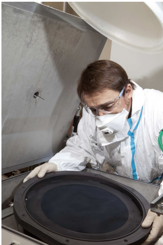
Fig. 5.9 Aligned carbon nanotubes after growth on a silicon wafer of 300 mm. This shows the output of the prototype reactor. Image courtesy of CEA/LETI (France)
