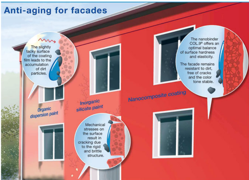
Fig. 21.9 Inorganic nanoparticles homogeneously incorporated in polymers provide ideal features for facade coatings. Image courtesy of BASF SE, Ludwigshafen
