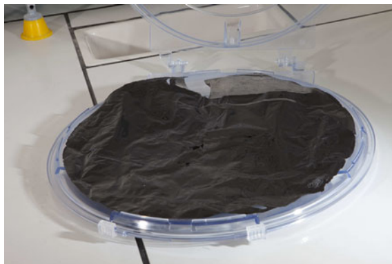
Fig. 5.10 Self-supporting carbon nanotube membrane obtained after removing the silicon wafer. It has a diameter of 300 mm and is obtained from the output shown in the Fig. 5.9. Image courtesy of CEA/LETI (France)
