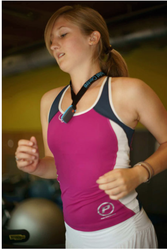
Fig. 17.6 Necklace for long-term and robust cardiac monitoring in sports life. Image courtesy Holst Centre (Netherlands)
