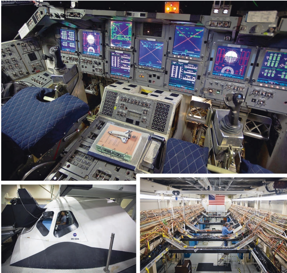
Fig. 7.6: [main] The cockpit of the Shuttle Avionics Integration Laboratory (SAIL) later in the Shuttle Program (showing the upgraded glass cockpit displays. [inset left] An exterior view of the SAIL. [inset right] The wiring feeds in the mock-up payload bay.
