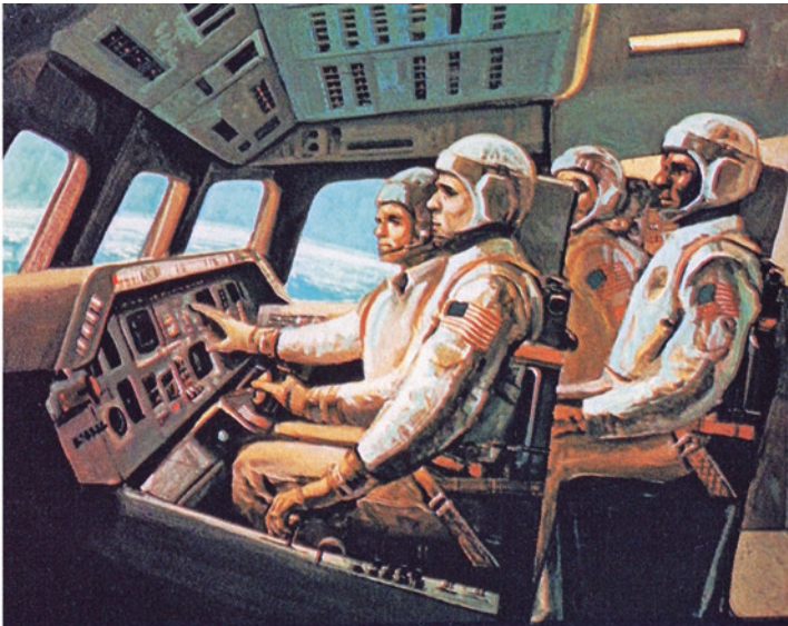
Fig. 2.6: The four-seat flight deck showing the pilots and Mission Specialists in their launch and (as shown here) entry positions. In this 1970s image, a multi-racial crew is evident, as is the lack of pressure suits.
