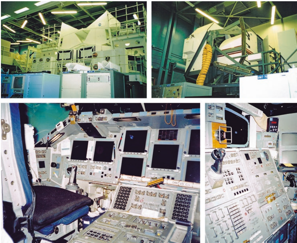
Fig. 8.3: (top pair) Space Shuttle Mission Simulator (SMS), Building 5, JSC. (bottom left) SMS Forward Flight Deck (Glass Cockpit). (right) SMS Aft Flight Deck (All images from the AIS archive).
