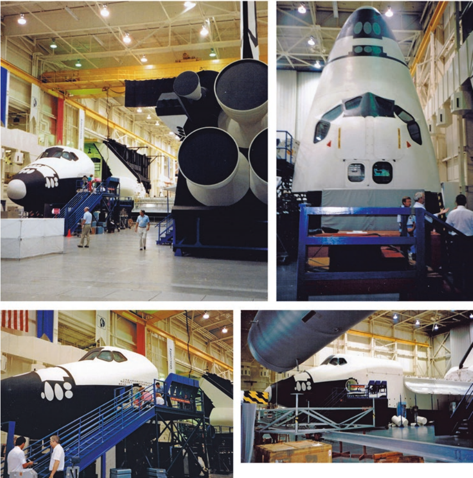
Fig. 8.4: [top left] Space Vehicle Mock-up Facility, Building 9, JSC. [top right] Crew Compartment Trainer. [bottom left] Forward Fuselage Trainer, [bottom right] 1G Full Fuselage Trainer (All images from the AIS archive).
