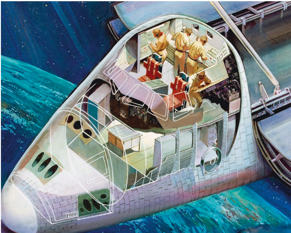
Fig. 2.5: 1970s cutaway image of the Orbiter crew compartment showing the upper flight deck and lower middeck living area.
