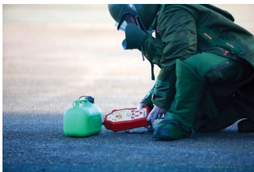
Figure 7.1. A handheld SORS spectrometer designed to detect hazardous materials. Source: © Agilent Technologies, Inc. 2016, 2018 Reproduced with Permission, Courtesy of Agilent Technologies, Inc.
