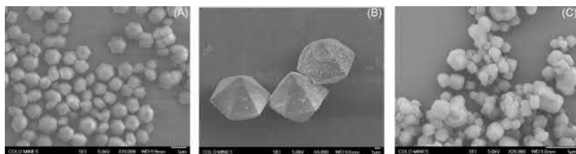
Figure 9.1 Representative SEM images of (A) Cu-MOF, (B) Ga-MOF, and (C) Al-MOF.
