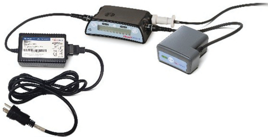
Figure 13.10. HVAD controller connected to one battery and AC power. Reprinted with permission from Medtronic, Inc.
