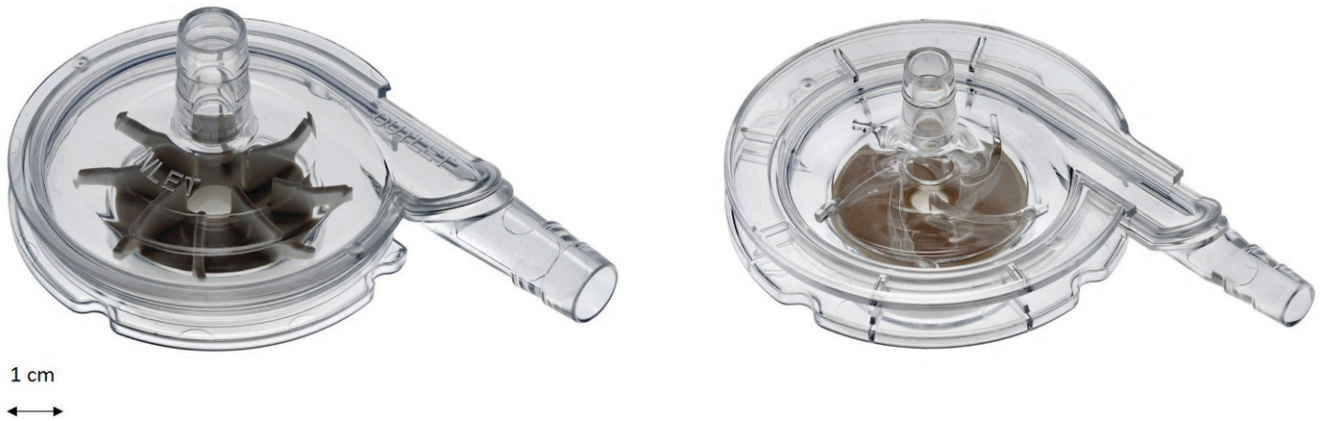
Figure 20.1. The CentriMag (left) and PediMag (right) blood pumps for adults and children, respectively. Each pump has a free-floating, magnetically levitated impeller that prevents it from contacting the pump housing, which reduces shear stresses that can cause blood trauma.
