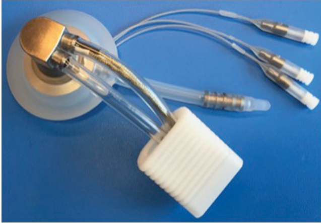
Figure 17.5. The NuPulseCV iVAS skin interface device (or SID). It has a wide base to adhere to the subcutaneous tissue for stability and a textured titanium neck for interfacing with the skin. The device has a microprocessor that digitizes the EKG and sends the signal to the driver. The SID acts as an electro-mechanical conduit for the EKG trigger and air. The cap can be rotated. The external driveline is attached to the patient with a connector.
