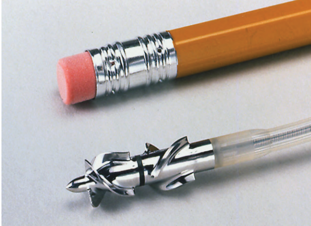
Figure 1.5. The Nimbus Hemopump impeller. Reprinted by permission from Springer Nature, Mechanical Circulatory Support: Principles and Applications , Morgan JA, Civitello AB, Frazier OH, eds., 2018.
