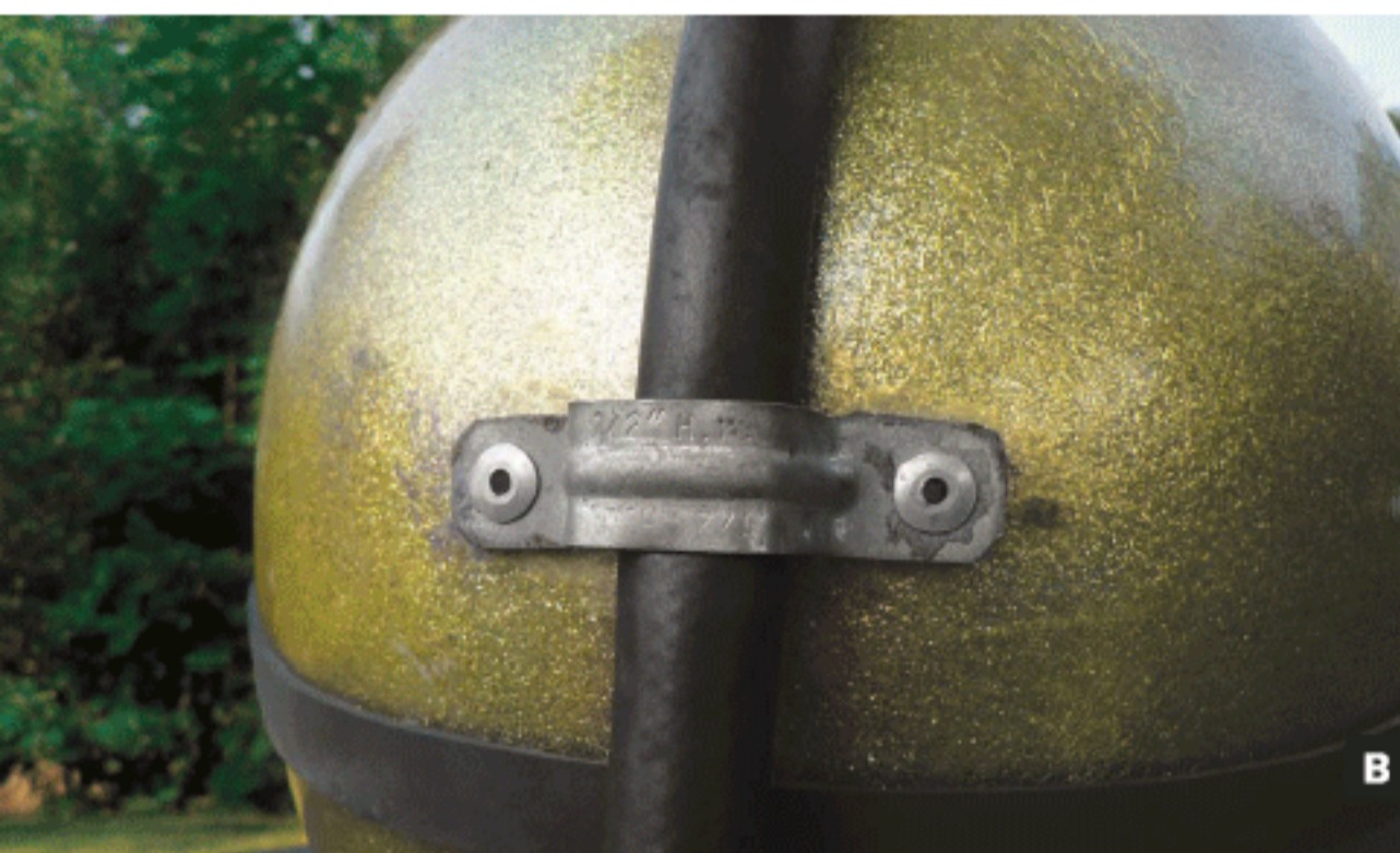
Fig. A: Bicycle brake cable snakes up from brake-lever trigger and threads through the extinguisher handles. Fig. B: Cable guide keeps the vinyl tubing in place at the base of the helmet.
