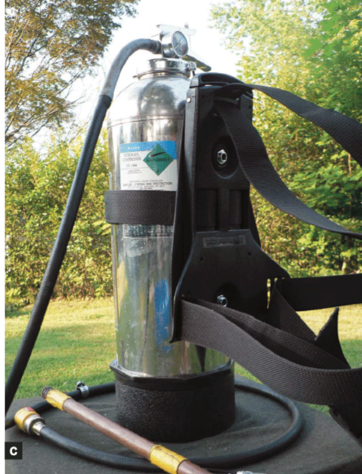
Fig C: Extinguisher, extender, backplate, and trigger rod are assembled and ready to go. Screw the garden hose quick-connect onto the helmet tube, and you're ready for combat.
