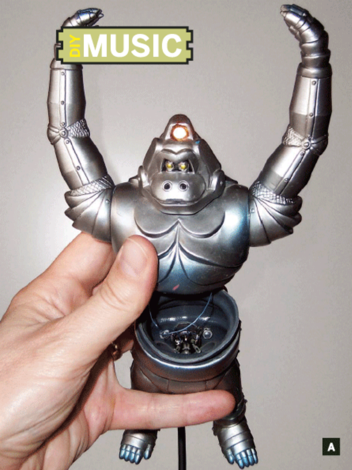
Fig. A: An LED between pins 4 and 5 on a MIDI Out or Thru jack will flash when data passes. Fig. A: When wiring a receptacle remember that the pins are reversed. You can also connect directly to a captive MIDI cable.
