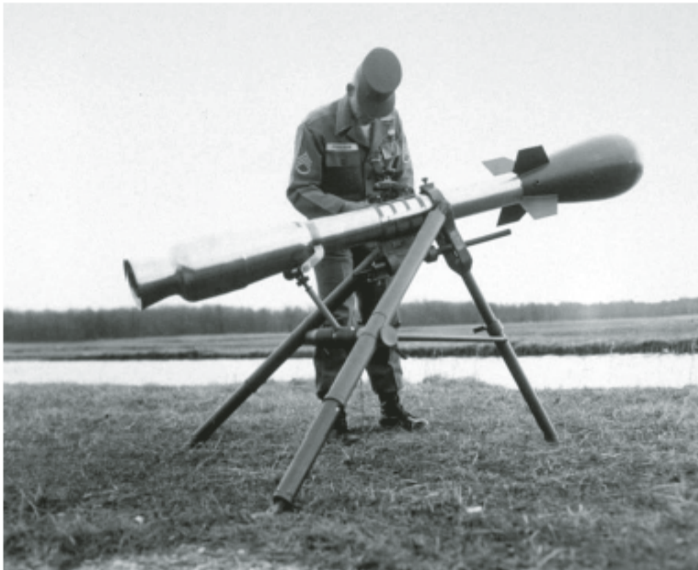
➔ The Davy Crockett, ready to be deployed. It had a warhead that was less than 12 inches in diameter, had a weight of about 60 pounds, and yielded up to a kiloton.
