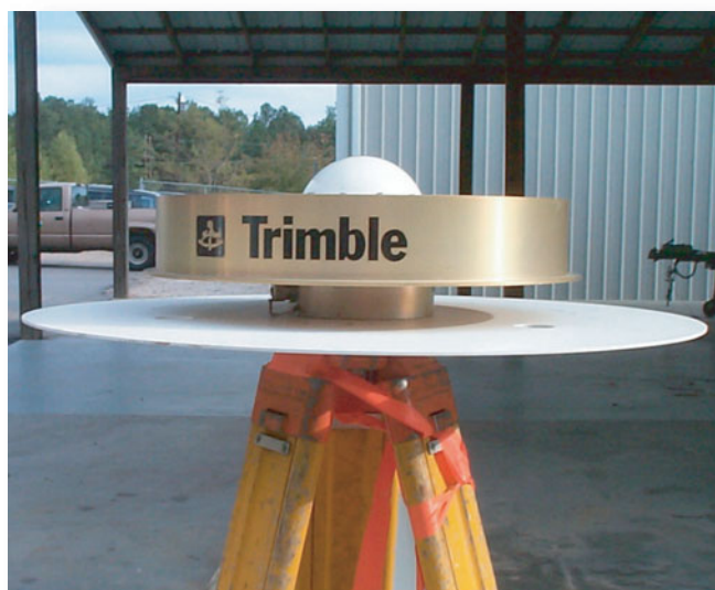
c. GPS receiver antenna that is placed on top of the tower.
