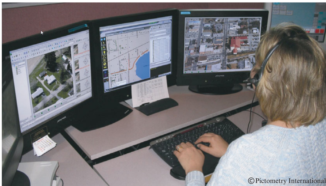
FIGURE 1-1 A 911 dispatcher receives an incoming call. Geospatial information stored in the GIS database is analyzed automatically to identify the geographic location of the caller. The dispatcher is then able to see the location of the caller on a digital map or digital aerial image as shown. In addition, the GIS may contain information about the current location of each of the potential first responders (e.g., police, fire, paramedics). The dispatcher or the GIS system then selects the responder that can reach the caller's location most efficiently (image courtesy of Pictometry International, Inc.).
