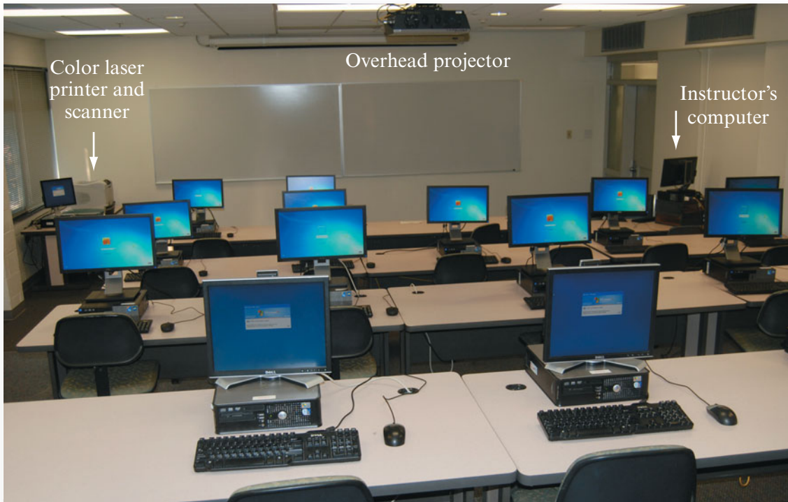
FIGURE 11-2 This typical GIS computer laboratory consists of multiple high-end personal computers with single, very fast CPUs, access to >5 TB of mass storage, high resolution computer screens (up to 1920 x 1080) with 512 MB to 1 GB of video memory, cursors, connection to a local area network (LAN), and access to the Internet. All of the computers have access to the color laser printer and scanner and to several devices not shown including a digitizing table and E-size inkjet plotter. The digital overhead projector allows the instructor to display items of interest and perform real-time GIS analysis.
