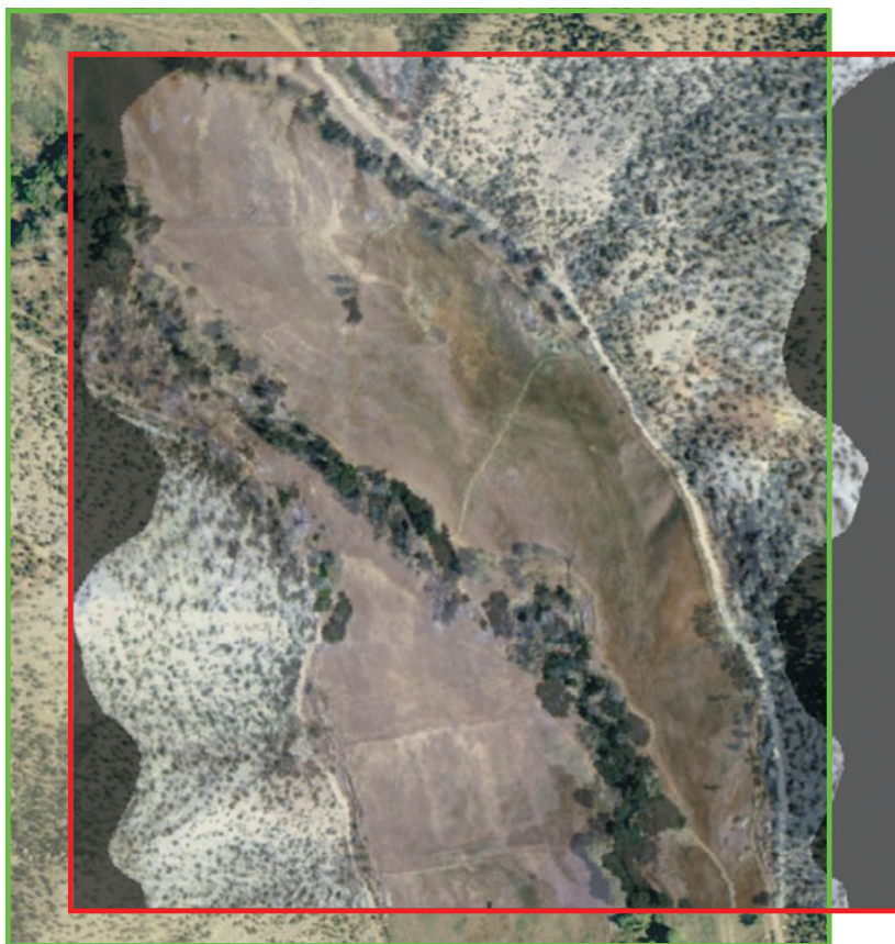
c. Geometrically corrected hyperspectral image overlaid on the reference image.
