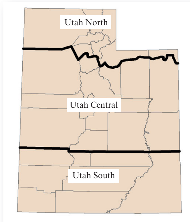
FIGURE 2-19 Each state has its own State Plane Coordinate System. The size and shape of each state determines the number of zones. Utah has three State Plane Coordinate zones (North, Central, and South) (data courtesy of ArcWorld Supplement and Esri, Inc.).
