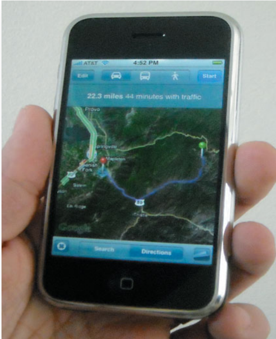
FIGURE 11-4 A cellular phone with navigation capability. The navigation capability is based on principles of GIS network analysis coupled with near real-time GPS positioning.
