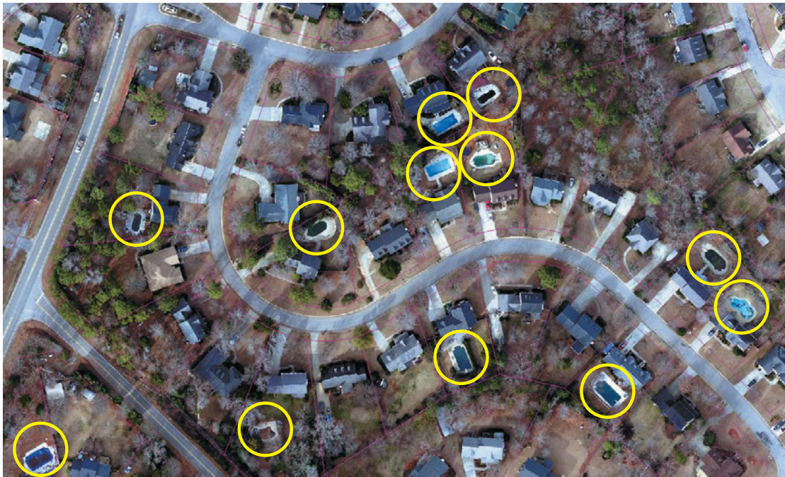
FIGURE 12-8 It is a straightforward task to identify the location of all the inground swimming pools using high spatial resolution aerial photography. The intersection of the location (address) of the swimming pools with a list of current swimming pool permits is an easy way to identify unpermitted pools (photography courtesy of Lexington County Property, Mapping and Data Services).
