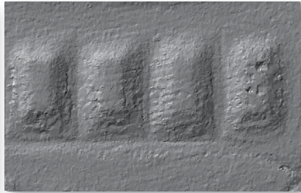
b. Analytically hill-shaded Triangular Irregular Network (TIN).
