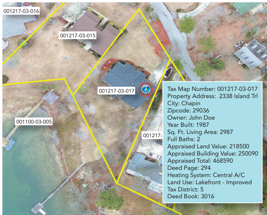
FIGURE 3-9 The surveyed parcel boundaries of the property at 2338 Island Trail, Chapin, SC, (tax map number 001217-03-017) are overlaid on 2011 natural-color vertical aerial photography. In developed countries, legal property boundaries associated with residential, commercial, and public property are almost always surveyed on the ground by a registered land surveyor. The attributes associated with a parcel are usually stored in a relational database (courtesy of Lexington County GIS Internet Property, Mapping, and Data Services).
