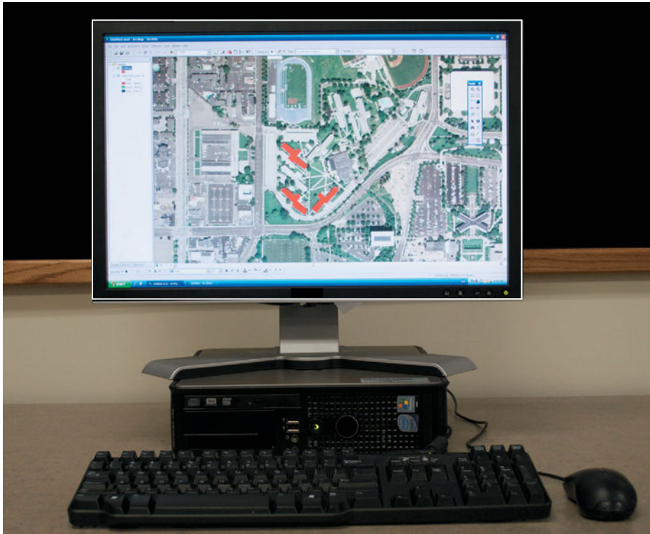
FIGURE 11-1 Properly configured personal computers and computer workstations are ideal for GIS analysis. In this example, the personal computer is being used to perform on-screen digitizing. A tracing device, such as keyboard direction keys or the mouse cursor and specialized GIS software, are being used to extract the coordinates of point, line, or area objects of interest. The outline (and area) of several large buildings (shown in red) have been extracted from the natural color orthophoto (data courtesy State of Utah).
