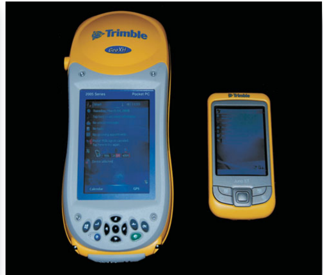
b. Two hand-held GPS receivers.
