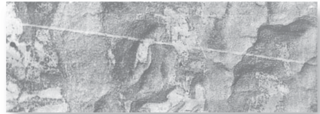
FIGURE 10-25 a) An uncorrected vertical aerial photograph of a power transmission line in rugged terrain. b) Planimetrically accurate orthophotograph after correction to remove roll, pitch, and yaw errors introduced by the aircraft at the instant of exposure and the effects of topographic relief displacement. Note that the transmission line is straight in the orthophoto (images courtesy of the U.S. Geological Survey).
