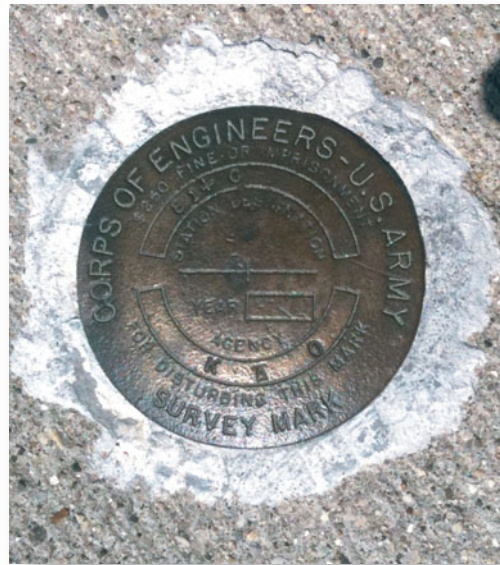
b. U. S. Army Corps of Engineers survey marker near Milwaukee, WI. 43° 02' 50.4" N latitude and 87° 52' 46.8" W longitude.
