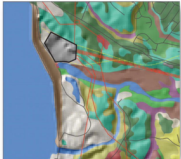
b. Removal of roads, powerlines, RR, and soil data within the extent of a polygon erase file. Hill-shaded DEM is allowed to show through for clarity.
