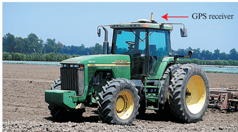
c. A GPS receiver installed on a tractor used for precision agriculture.
