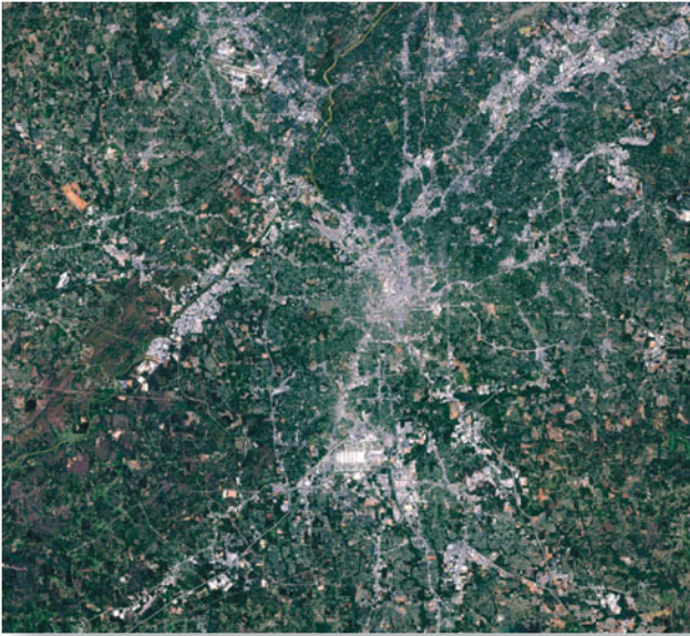
a. Landsat 7 Enhanced Thematic Mapper Plus (ETM + ) image obtained on September 28, 2000 (RGB = bands 3,2,1; 30 x 30 m pixels).
