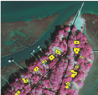
a. Point (building centroids), line (road network), and area (building footprint) features.
