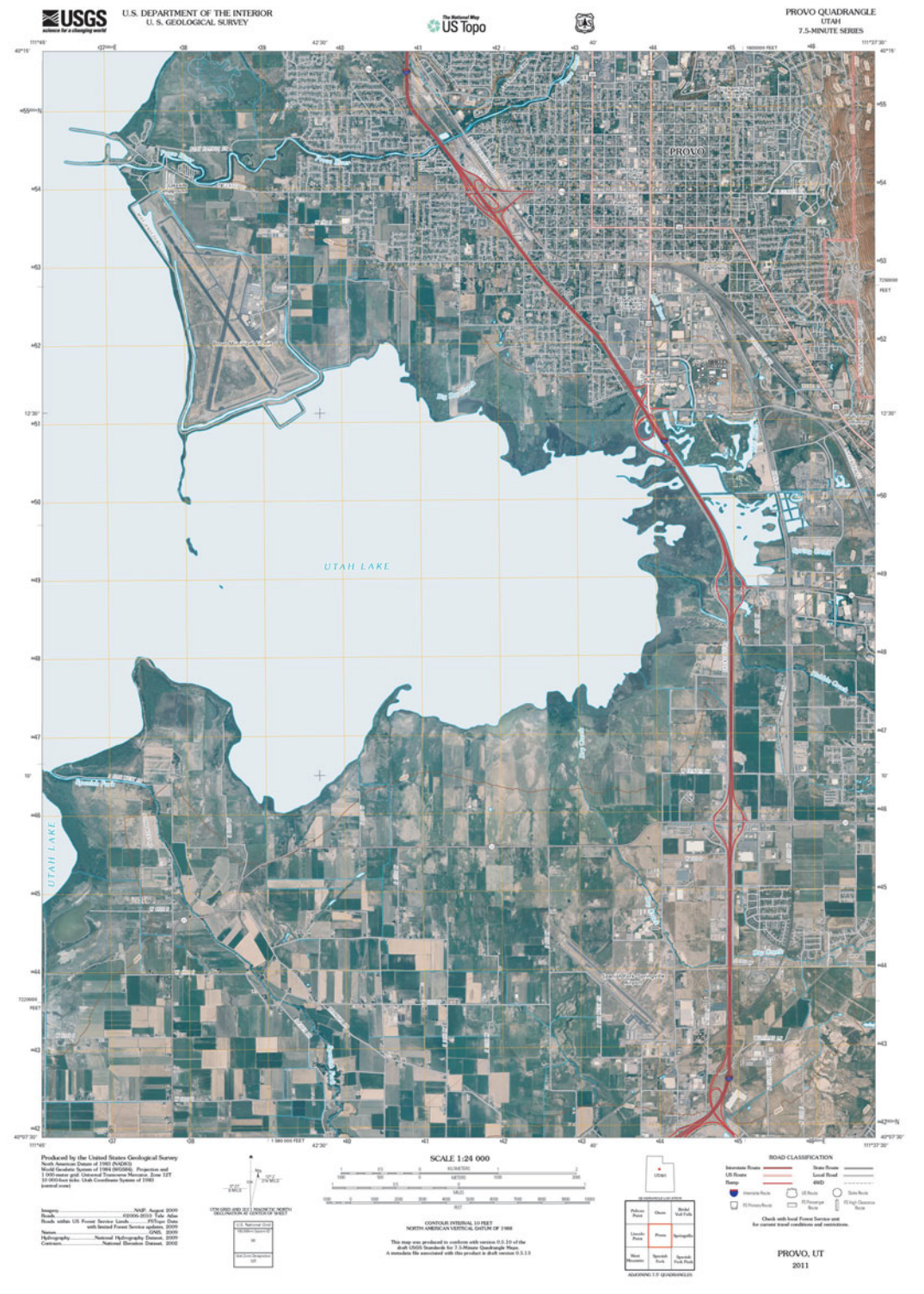
FIGURE 1-8 The U.S. Geological Survey’s National Map program provides quantitative geospatial information for input to a GIS. This example is a US Topo GeoPDF of the Provo, UT, 7.5-minute quadrangle with elevation data from the National Elevation Dataset (NED), hydrology data from the National Hydrology Dataset (NHD), and aerial photography from the National Agriculture Imagery Program (NAIP). The US Topo information can be viewed using a PDF viewer. The spatial information can be downloaded directly from The National Map website (data courtesy of the U.S. Geological Survey).
