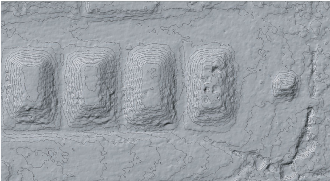
b. LiDAR-derived bare-Earth digital terrain model overlaid with 25 cm contours.
