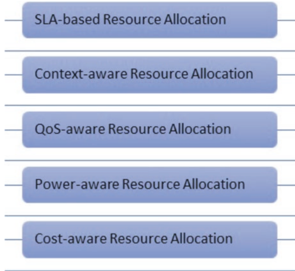
Fig. 4.6 Classification of IoT resource allocation techniques
