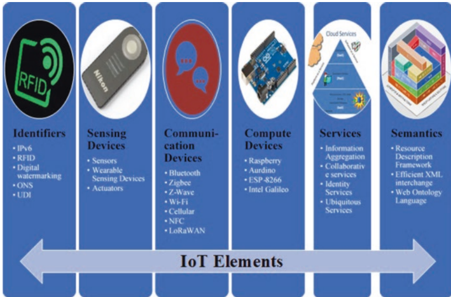
Fig. 4.1 Basic elements of the IoT environment
