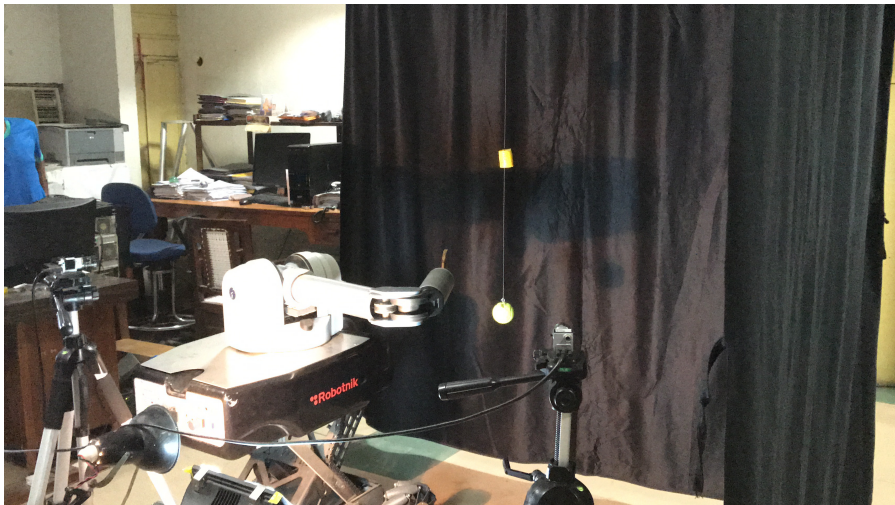
FIGURE 2.9: Hardware setup consisting of two off the shelf cameras, a hanging ball and 4 DOF Barrett Wam Robot Manipulator.
