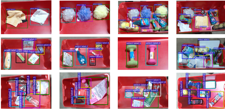
FIGURE 10.23: A few example images of the automatic ground truth detection results when objects are placed in varying degree of clutters. The annotation model detects ROI and end-user can write a label on each detected ROI for further categorization of objects. The clutters contain both a known set of objects as well as unknown objects.
