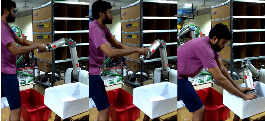
FIGURE 1.8: A robotic manipulator is given kinesthetic demonstrations for pick and place task.
