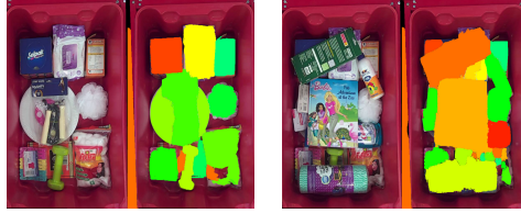
FIGURE 10.28: A few examples of the automatic segmentation results when tested in a real-world cluttered environment as shown here. It is important to note here that the training dataset contains only synthetically generated clutters.
