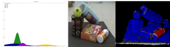
(b) Use of GMM model using both color and depth curvature information
