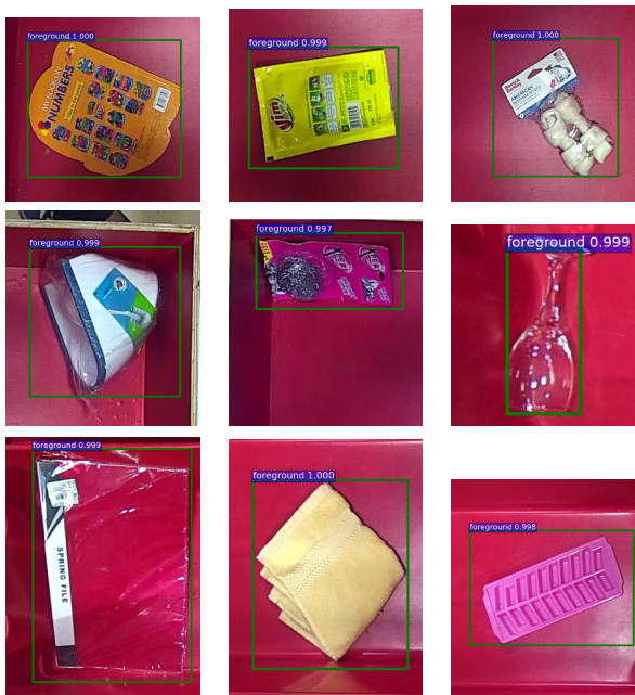
FIGURE 10.21: Automatic annotation results of few images when tested on same background using an entirely new set of objects. These objects were never shown to the model previously.
