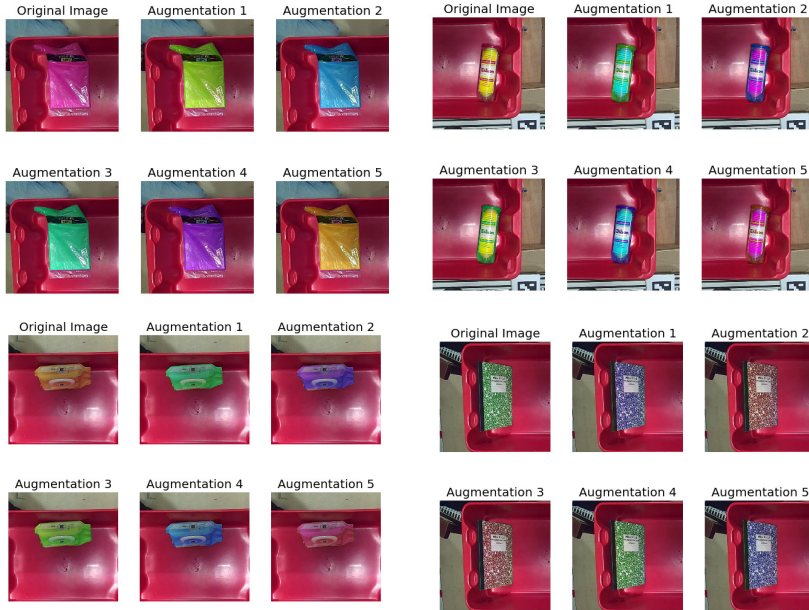
FIGURE 10.18: Example images showing color augmentation results. Color augmentation increase the data size five times to its original size.
