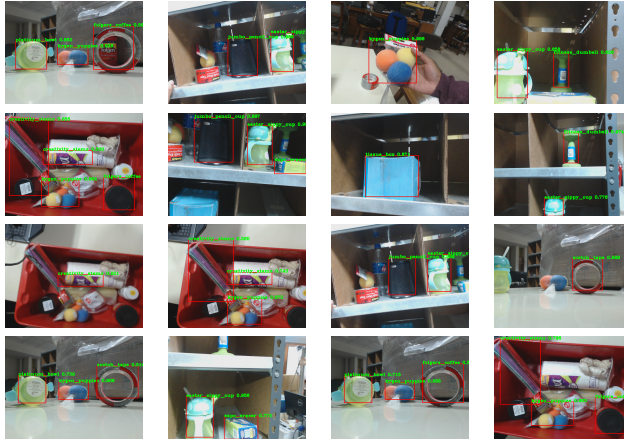
FIGURE 12.24: Output of RCNN after training. The objects are detected in different environments (different backgrounds). Each recognized object is provided a label and a bounding box.
