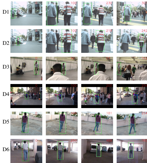
FIGURE 16.16: Tracking results for different datasets. The green window is the main tracking window for the target being tracker while white window is the estimated target location obtained from a predictor.
