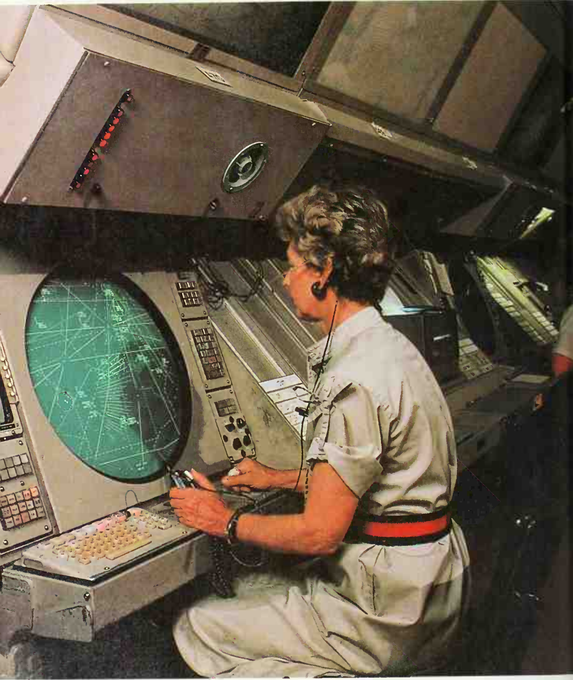
Air traffic controllers use radar to direct planes near busy airports. The moving spots of light on the radar screen show where each plane is.
