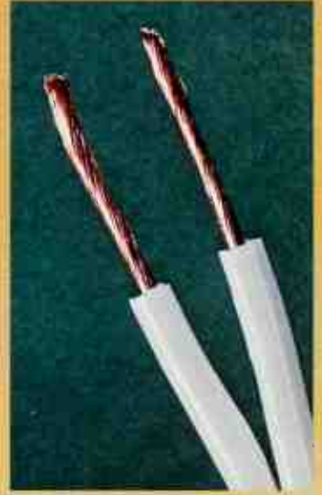
The metal part of the wire carries electricity. The rubber or plastic covering keeps the electric current from leaving the wire.
