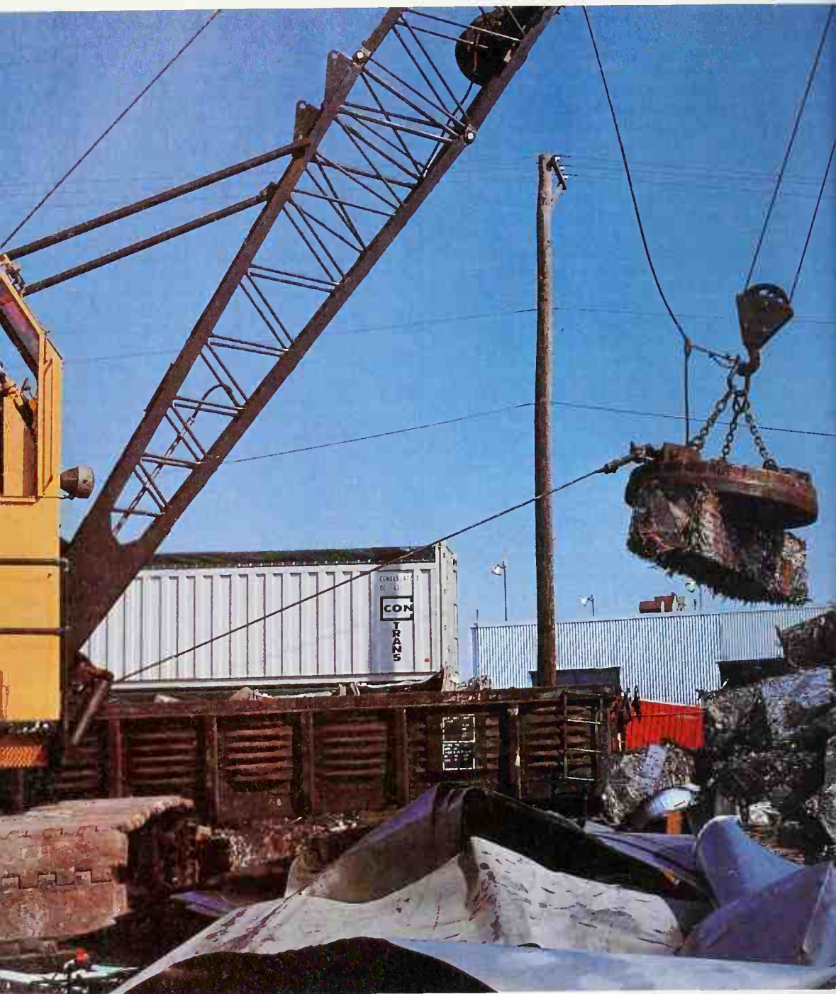
Large electromagnets can lift heavy loads. This one picks up and stacks big blocks of crushed iron and steel in a junkyard.
