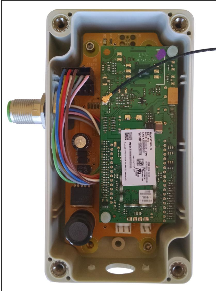
In the preceding diagram, the lower circuit board implements the functionality of the device (monitoring cryogenic liquids, in this case). On this board, the power supply system, sensor electronics, and a low-cost, 16-bit microcontroller are found. A cellular modem is located on the top circuit board, which plugs into a socket on the lower board.
