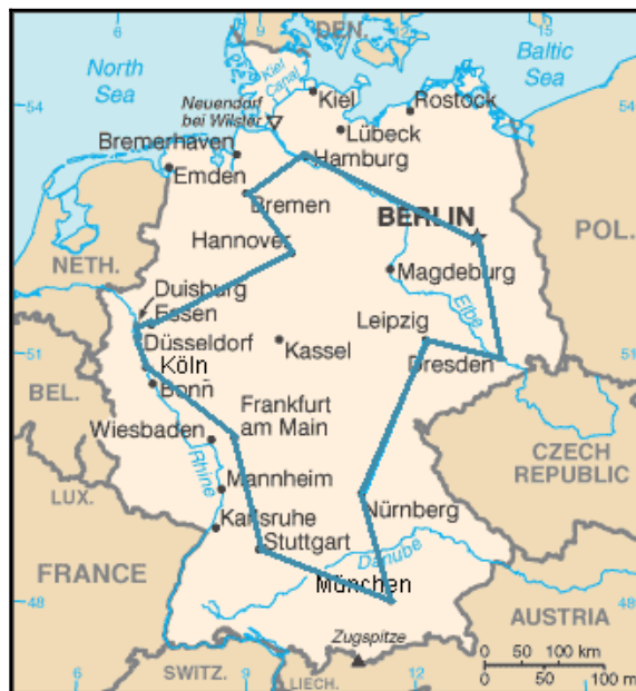
The shortest TSP path for the 15 largest cities in Germany Source: https://commons.wikimedia.org/wiki/File:TSP_Deutschland_3.png Image by Kapitän Nemo. Released to public domain
