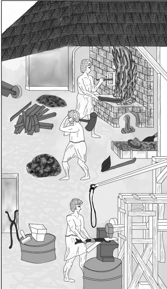
Figure 6.3 Forging the bloom.
