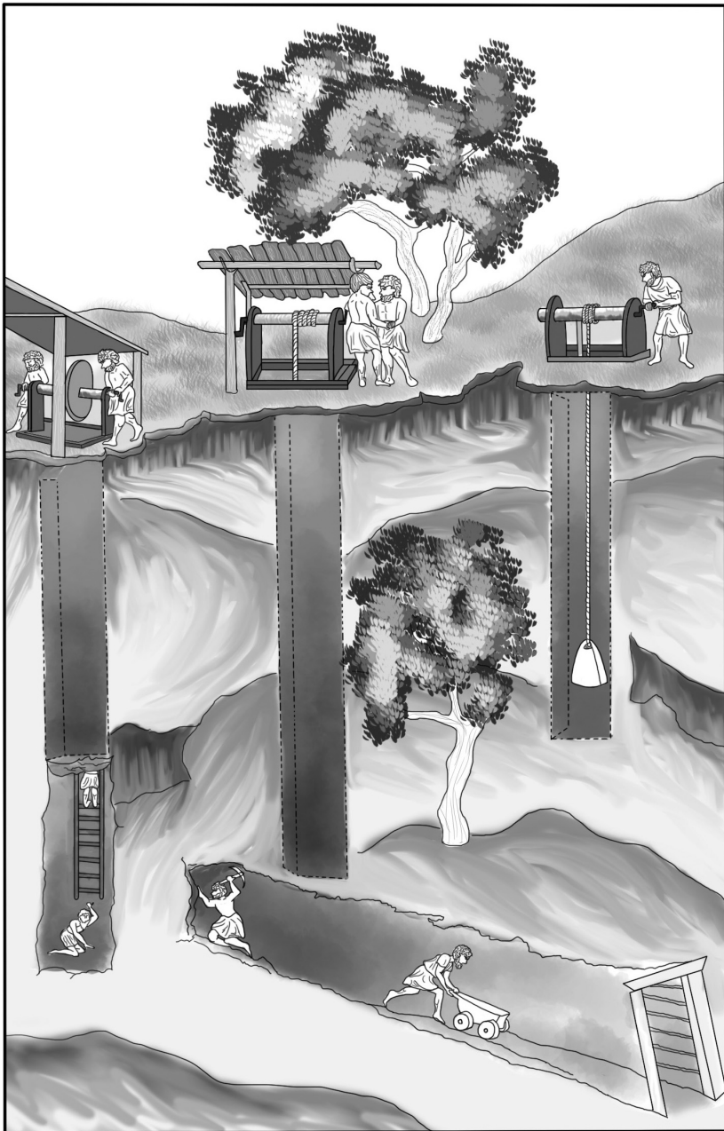
Figure 5.2 The arrangement and operation of mining shafts.
