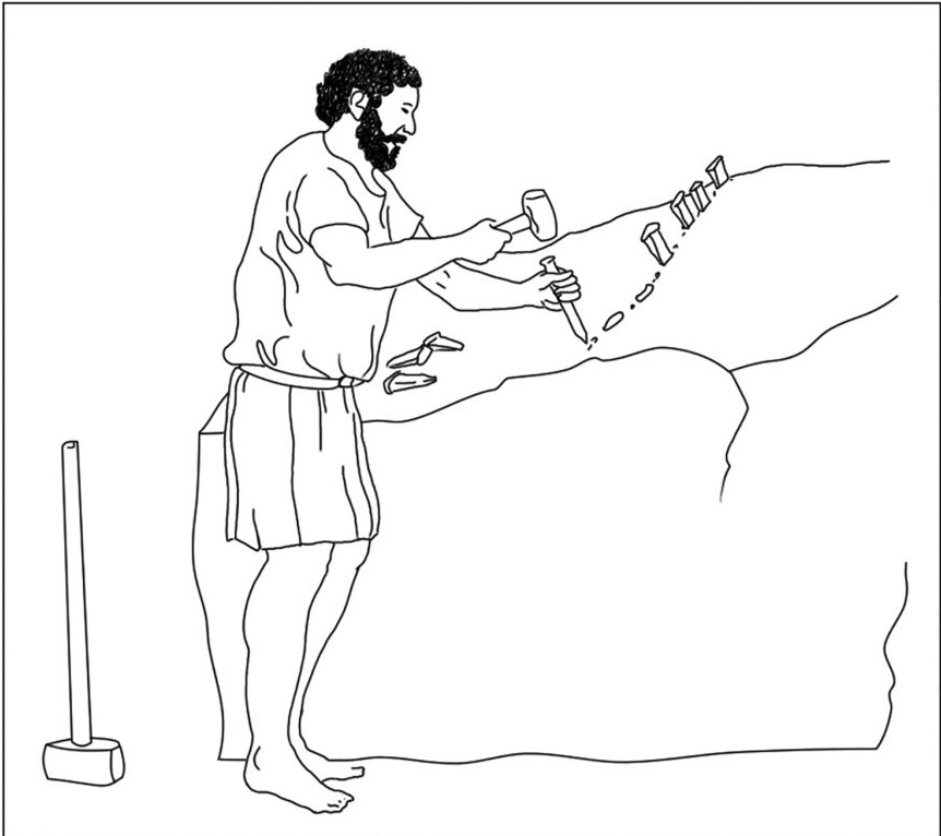
Figure 5.7 Splitting a rock with wedges.
