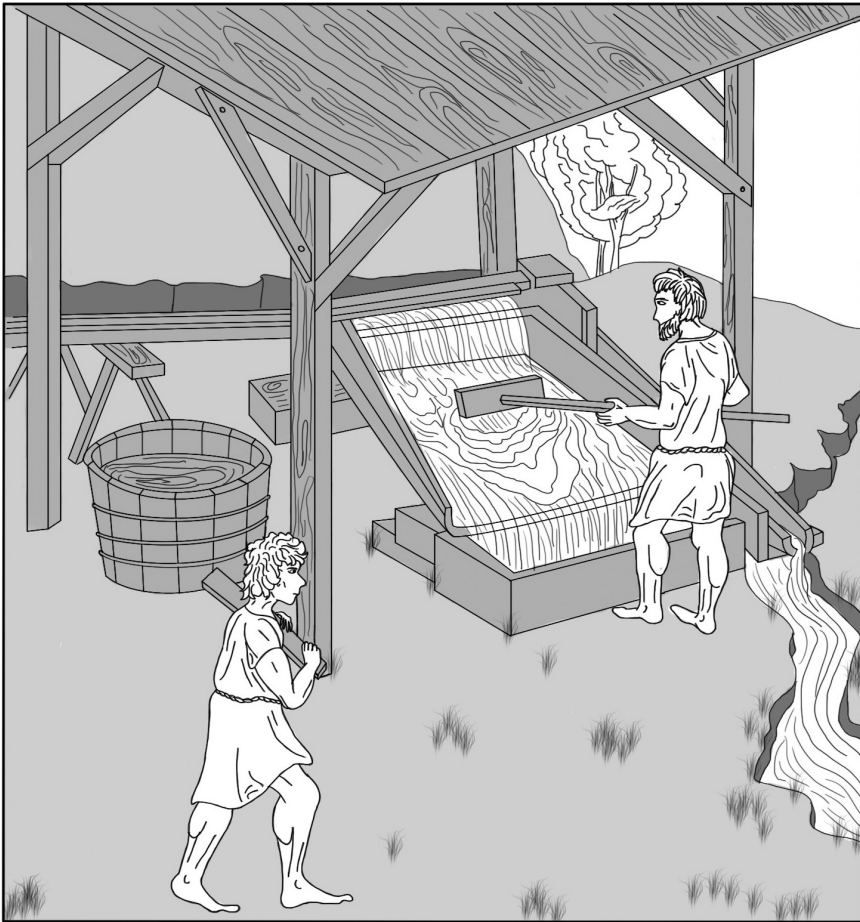
Figure 6.2 Washing the ore.
