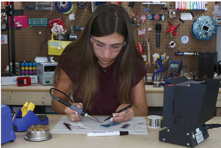
FIGURE 5-1: Soldering an SMD with a standard soldering iron.
