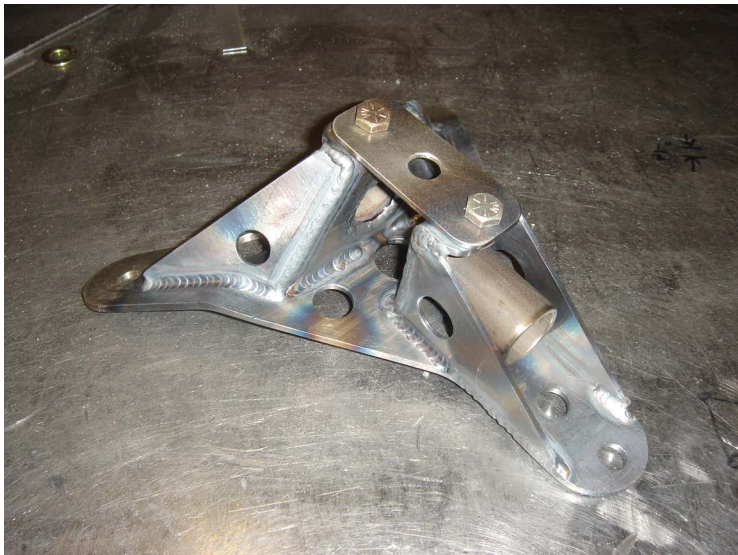
FIGURE 1-7: A welded connector for an off-road vehicle IMAGE COURTESY OF ROCK BUG BUILD ALBUM, FLICKR COMMONS, LICENSED UNDER CC BY 2.0
