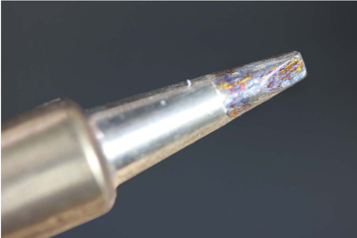
FIGURE 3-3: A dirty soldering iron
