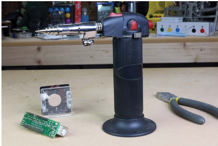
FIGURE 2-14: Gas-fueled soldering iron
