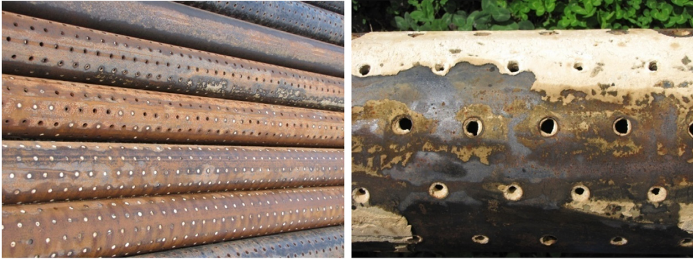
Figure 9.15 Silica scaling in reinjection well perforated liner showing many blocked perforations due to silica scaling (pictures by authors).
