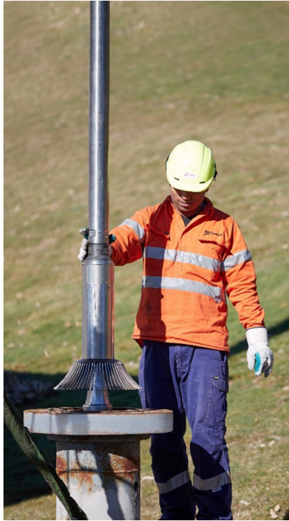
Figure 7.13 Mechanical calliper showing the extended multiple fingers. With kind permission from MB Century Ltd.
