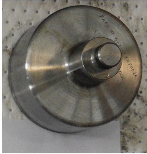
Figure 7.14 Lead impression block 5½" diameter. With kind permission from MB Century Ltd.
