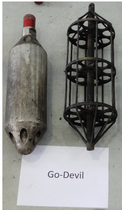
Figure 7.4 Common designs of go-devils (aluminium on the left, brass on the right) used by the geothermal industry. From MB Century Ltd., with kind permission.
