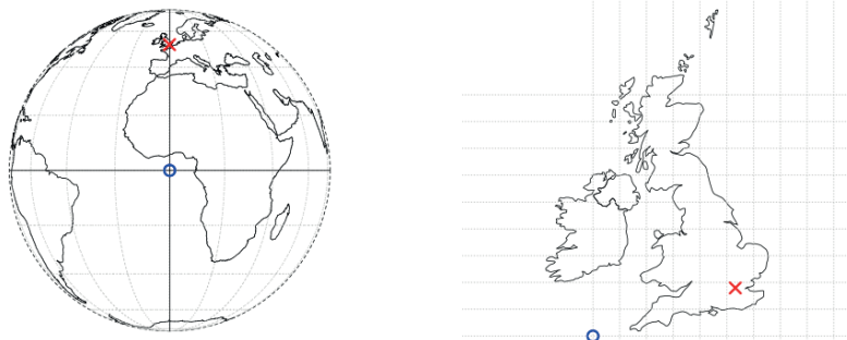
FIGURE 2.1: Illustration of vector (point) data in which location of London (the red X) is represented with reference to an origin (the blue circle). The left plot represents a geographic CRS with an origin at 0^\circ longitude and latitude. The right plot represents a projected CRS with an origin located in the sea west of the South West Peninsula.
