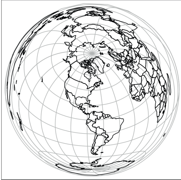
FIGURE 6.5: Lambert azimuthal equal-area projection of the world centered on New York City.
