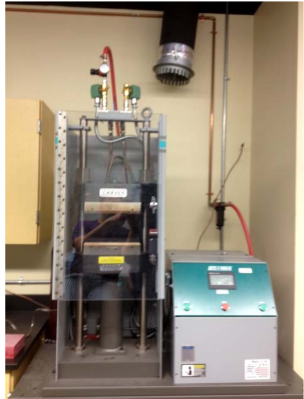
Figure 2.7 An automatic hydraulic uniaxial press for bulk ceramic processing (Carver Company). Source: Courtesy of Electroceramics Lab. at Ingram School of Engineering at Texas State University, San Marcos, TX.
