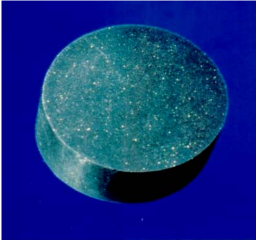
Figure 2.8 A sample of 123 YBCO ceramic superconductor. Source: Courtesy of Electronic Materials Laboratory, ECE Department, Texas A&M University, TX, ca. 1988.
