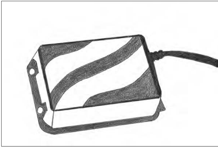
Figure 6-2: An air pump adds bubbles to the water, helping gas exchange at the surface.
